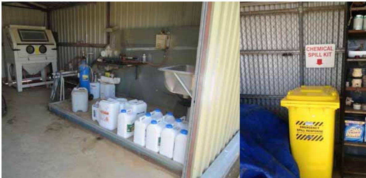
**Figure 6: Appropriate bunding and a spill kit in chemical storage areas**
