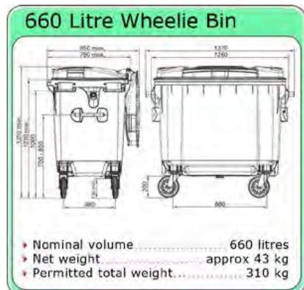
Figure 37 Typical 660 litre bin specifications
