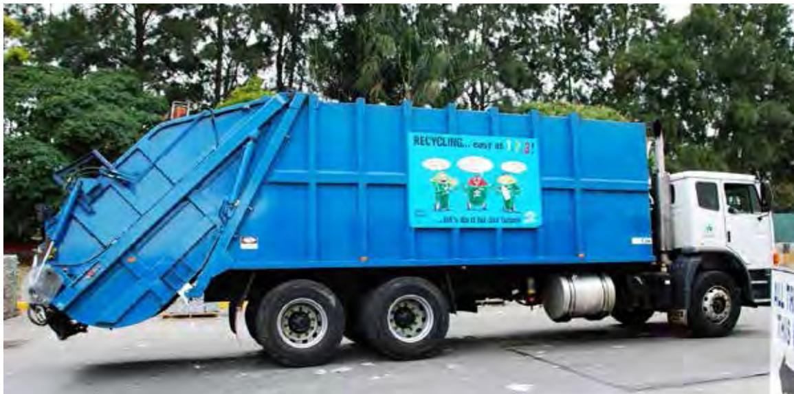
Figure 57 A rear-lift collection vehicle
