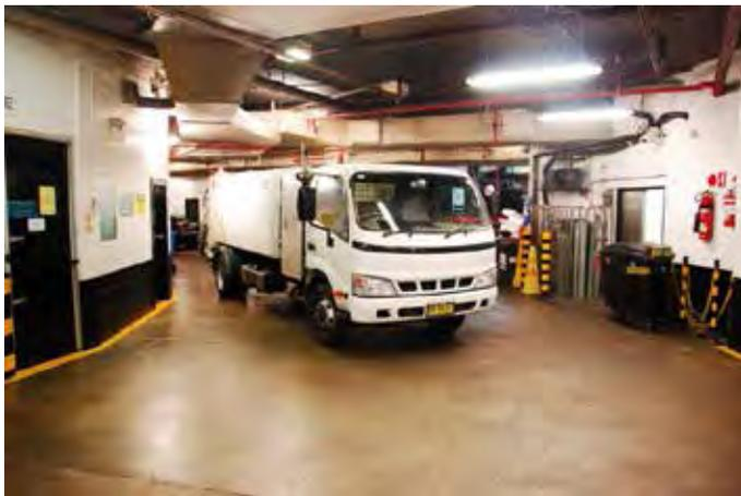
Figure 21 Small vehicle for access to areas with low clearance
