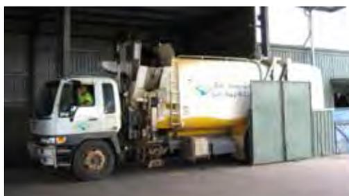
Figure 32 Side-lift collection vehicle
