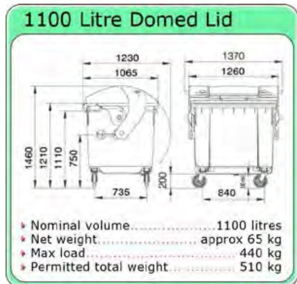
Figure 39 Typical 1100 litre bin specifications
