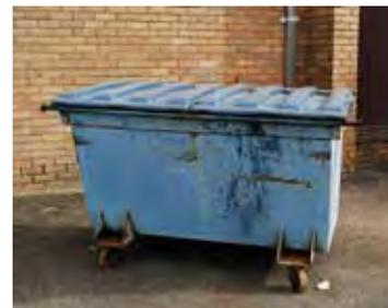
Figure 26 Rear-lift bulk bin
