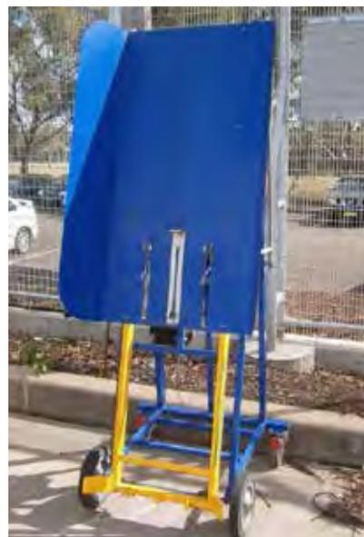
Figure 50 A simple gas strut bin lifter
