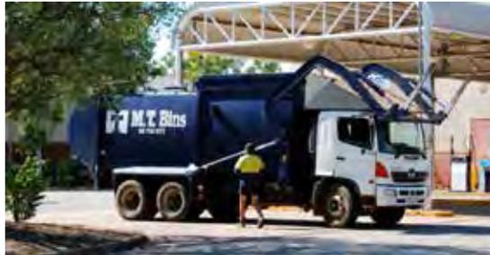
Figure 29 Front-lift truck
