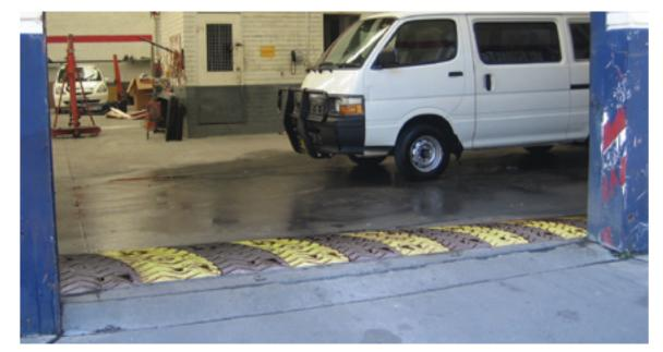
If the workshop walls and floor are well sealed, the workshop can be bunded with a small concrete speed hump (or flexible rubber hump) across all doorways.
