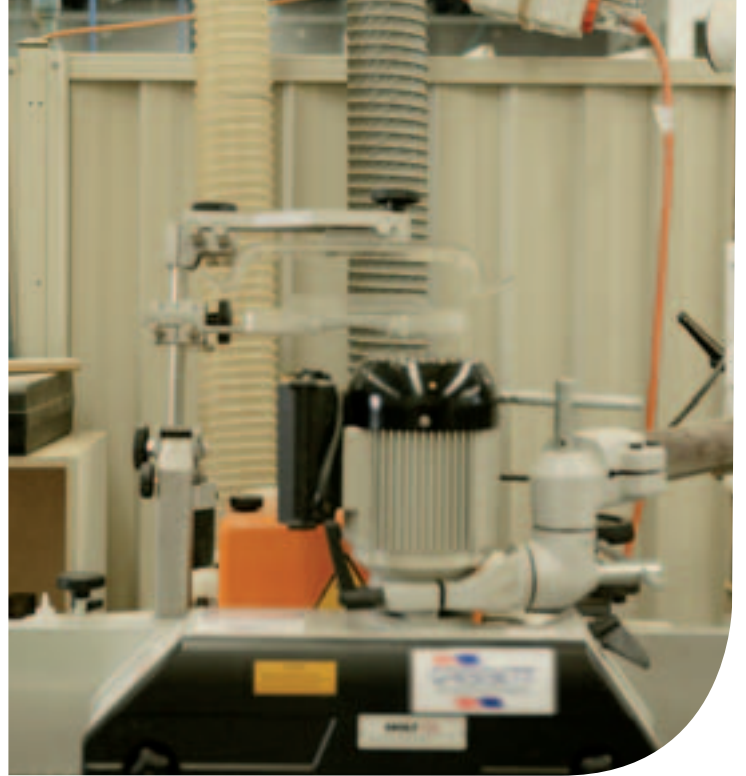
Connecting equipment to a dust extractor is the easiest way to control dust.
