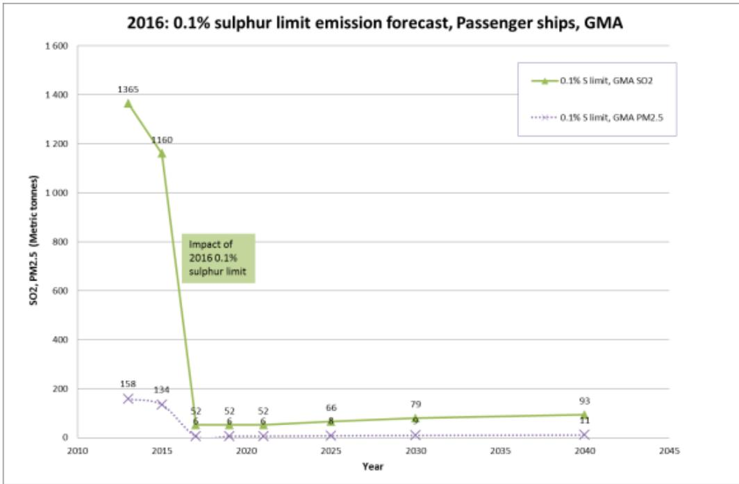
Figure 7-45: Predicted passenger ship emissions in the GMA if 2016 0.1% S limit
