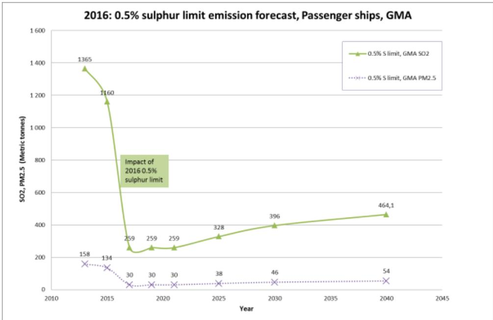
**Figure 7-41: Predicted passenger ship emissions in the GMA if 2016 0.5% S limit**
