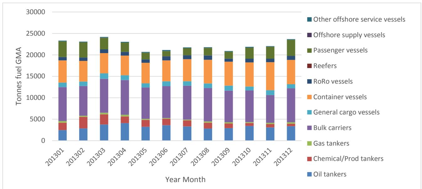
**Figure 7-5 Monthly variations of fuel consumption in the GMA for main engines, auxiliary engines and boilers**
