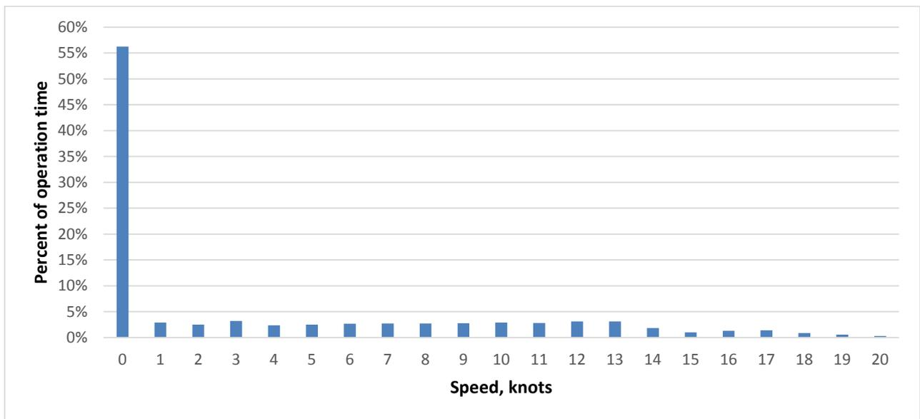
Figure 7-9 : Passenger cruise vessels speed profile in the GMA – 2013 data
