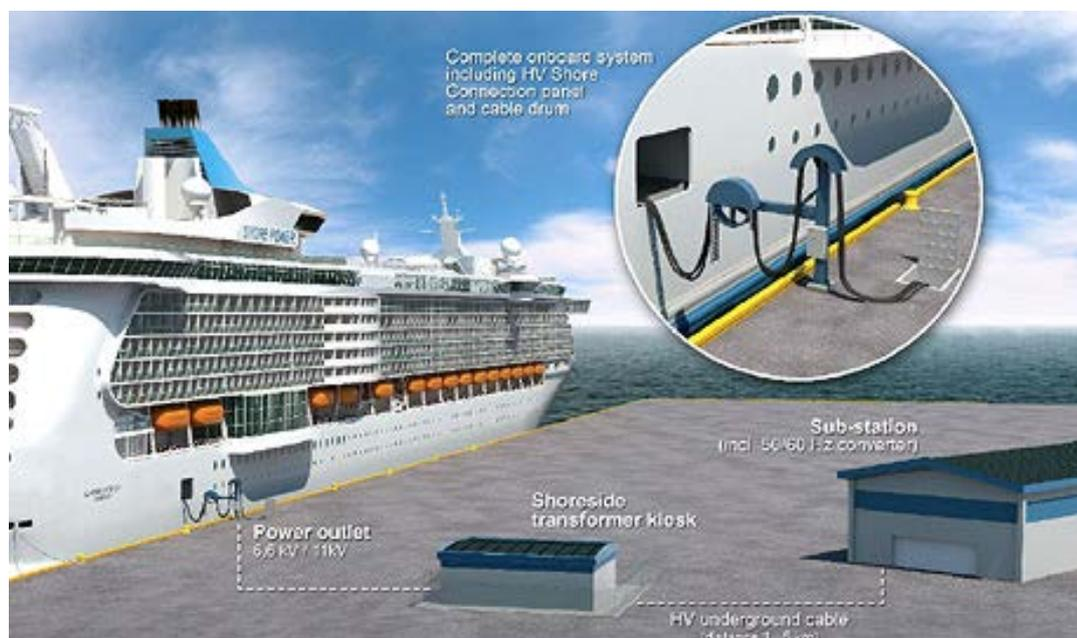
Figure 4-4: Typical shore side power system layout<sup>24</sup>
