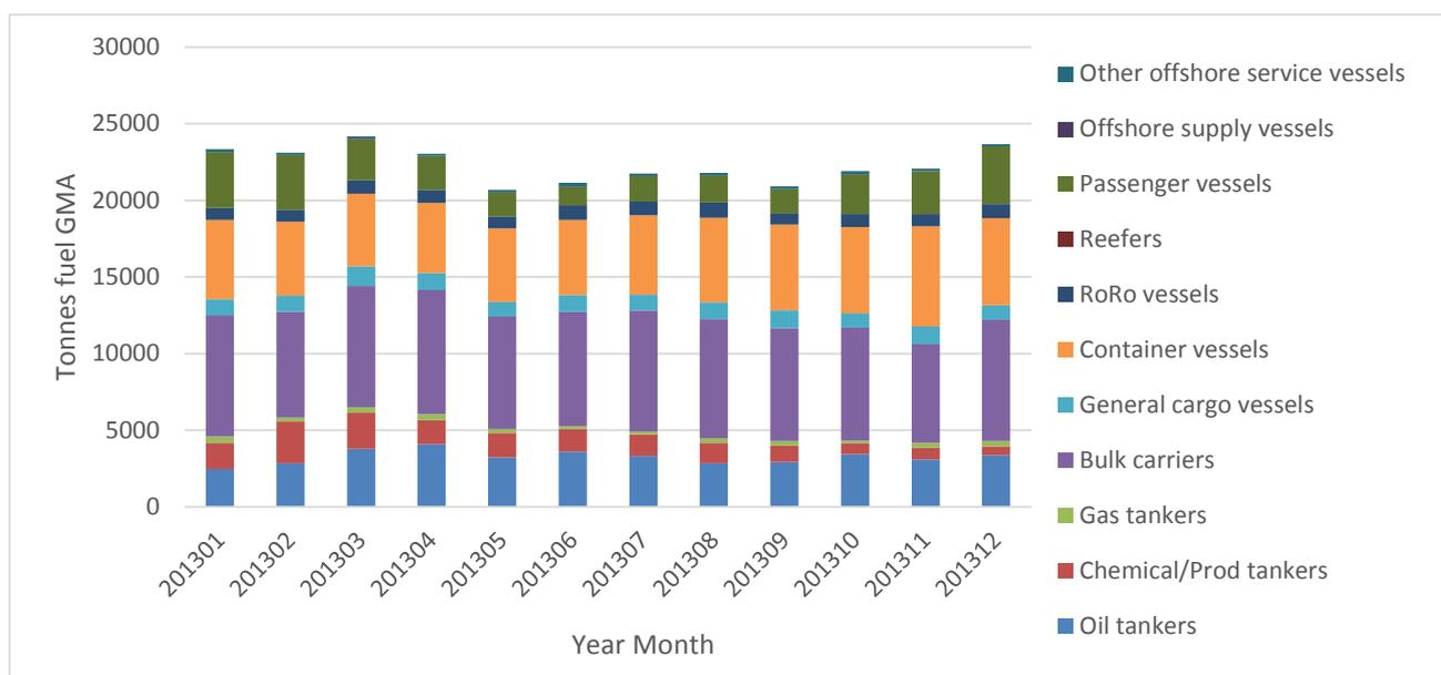
Figure B: Fuel consumption by main ship types for all identified ships in the GMA, monthly, 2013
