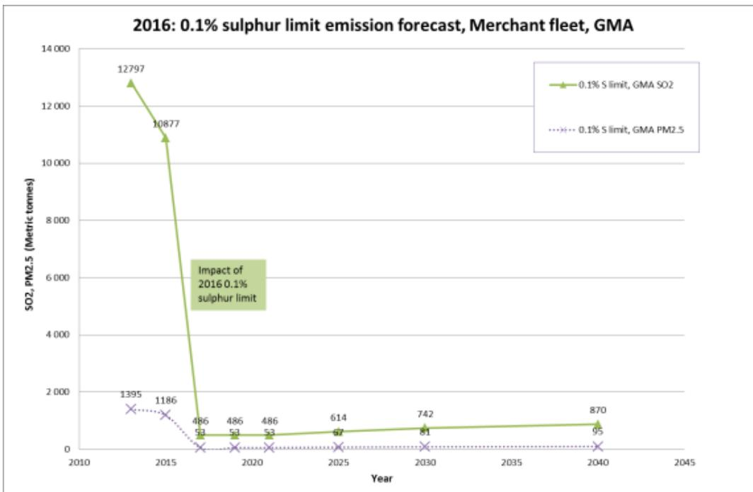
Figure 7-46: Predicted merchant ship emissions in the GMA if 2016 0.1% S limit
