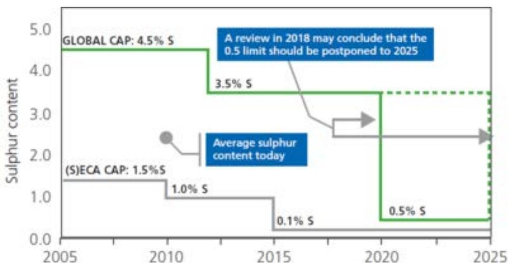
Figure 5-2: Timeline for restrictions on sulphur content (IMO 2011)<sup>38</sup>
