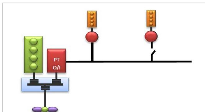
**Figure 4-1: Main engine with connected generator and two auxiliary engines**
