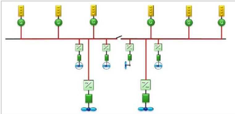
**Figure 4-2: Typical diesel-electric engine configuration**
