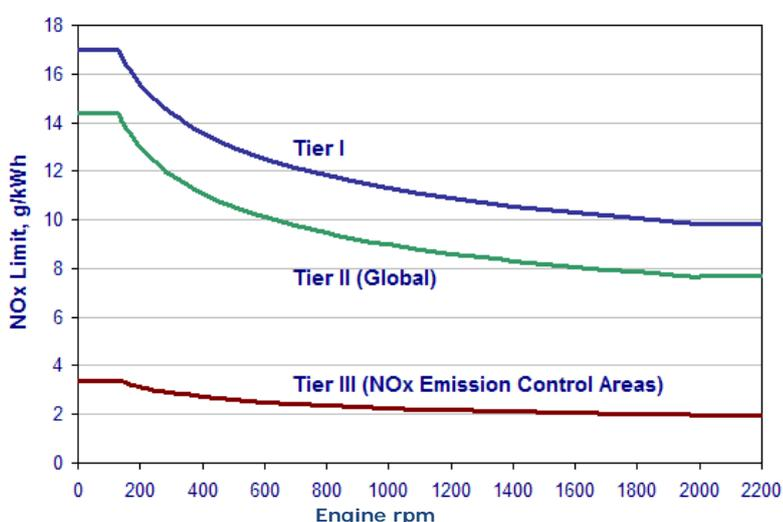
**Figure 5-4: IMO NOx regulations, for all ships with engine of over 130 kW output power**
