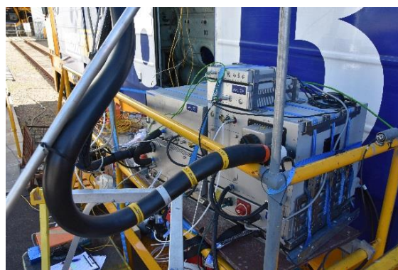
Gaseous heated sample entry to PEMS
