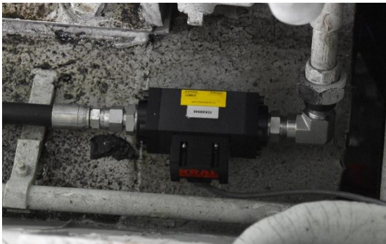
High precision fuel flow meter on delivery line
