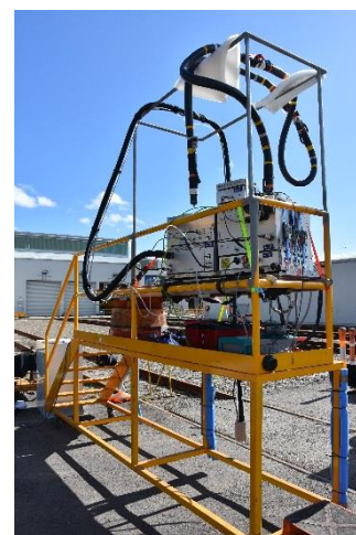
PM and Gas PEMS set up prior to the locomotive arriving
