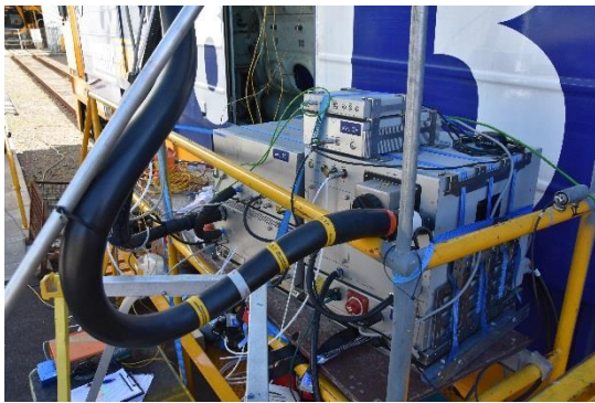
PEM system and emissions sample lines
