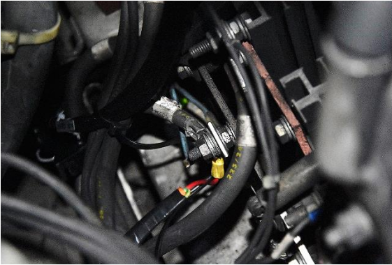
Voltage connections for auxiliary DC generator
