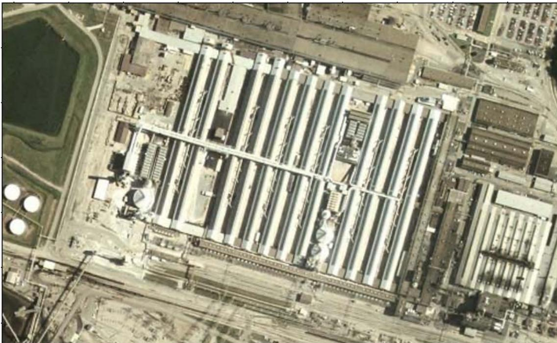
**Figure 3-2. Aerial photograph of a typical aluminum plant showing rows of potrooms.**
