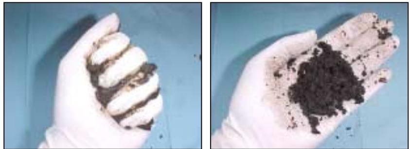
**Plates 23 and 24.** Sample too wet for vermiculture processing (left and right). The sample deforms significantly after the fist is opened, does not fall apart when pressure is applied or if a large amount of water is released, the sample is too wet for vermiculture processing (right).
