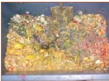
Plate 4 shows a final feedstock of size reduced fruit and vegetables blended with a cardboard bulking agent.
