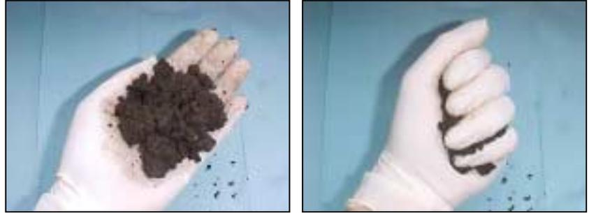
**Plates 21 and 22.** Sample with suitable moisture content for vermiculture processing glistens slightly - some water released between the fingers (left). Sample too dry for vermiculture processing (right). Sample crumbles without further action when the fist is opened.
