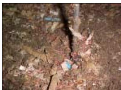
**Plate 17.** Scrape back the interface between the feedstock layer and bedding material (Zone 2 on Figure 3 above).
