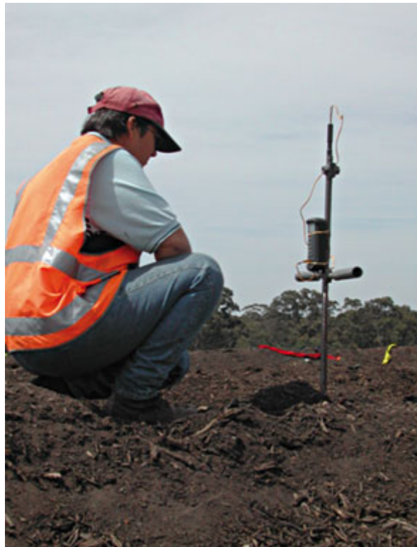
Figure 14. Illustration of the temperature probe used to monitor the temperature of the windrow at 0-15, 50-75 and 100-150cm depths.
