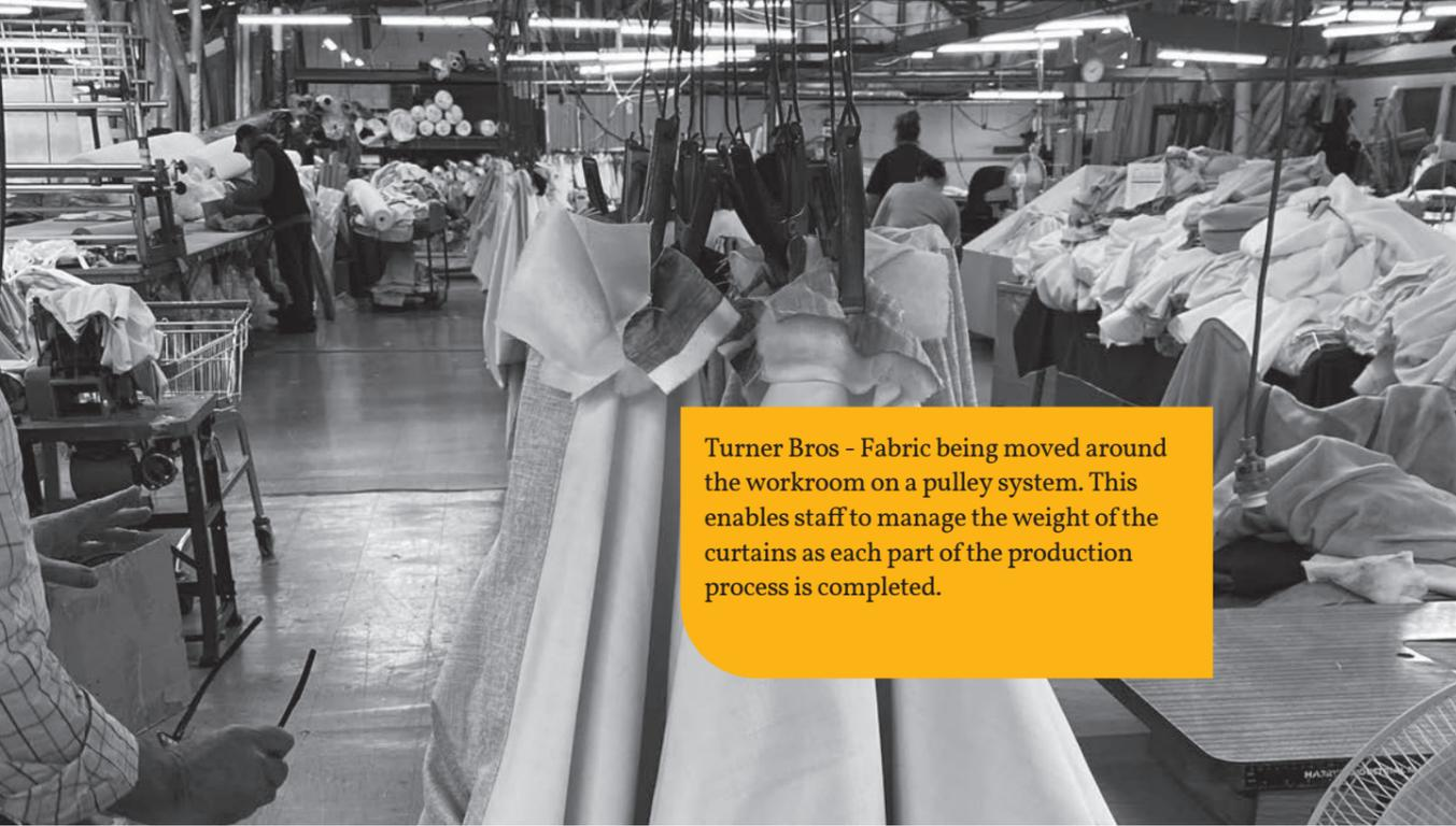
Turner Bros - Fabric being moved around the workroom on a pulley system. This enables staff to manage the weight of the curtains as each part of the production process is completed.
