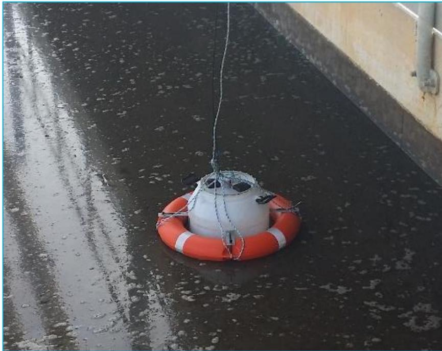
Figure 5.7. Floating flux chamber in use at a sewage treatment plant
