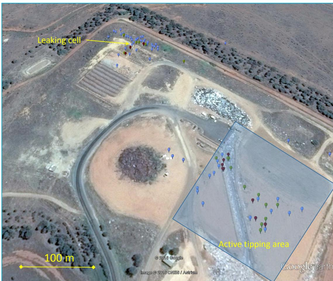
**Figure 6.28. Parkes Waste Facility showing the locations where flux chamber measurements were made within the active area of the facility. This is a compilation of measurements made during four separate site visit. The blue markers represent low emissions ( $< 1 \text{ g CH}_4 \text{ m}^{-2} \text{ day}^{-1}$ ), Green markers intermediate ( $1 \text{ to } 10 \text{ g CH}_4 \text{ m}^{-2} \text{ day}^{-1}$ ) and red are high emissions ( $>10 \text{ g CH}_4 \text{ m}^{-2} \text{ day}^{-1}$ ).**
