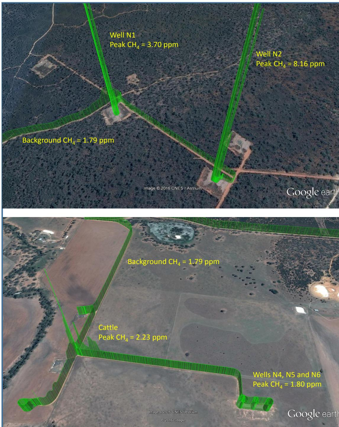
**Figure 6.23. Mobile surveys of CH<sub>4</sub> concentration in the vicinity of Wells N1, N2, N4, N5 and N6 made during February 2016. The maximum CH<sub>4</sub> concentration (dry basis) of peaks and background are indicated. Note the magnitude of the peaks associated with cattle grazing near Wells N4, N5 and N6.**
