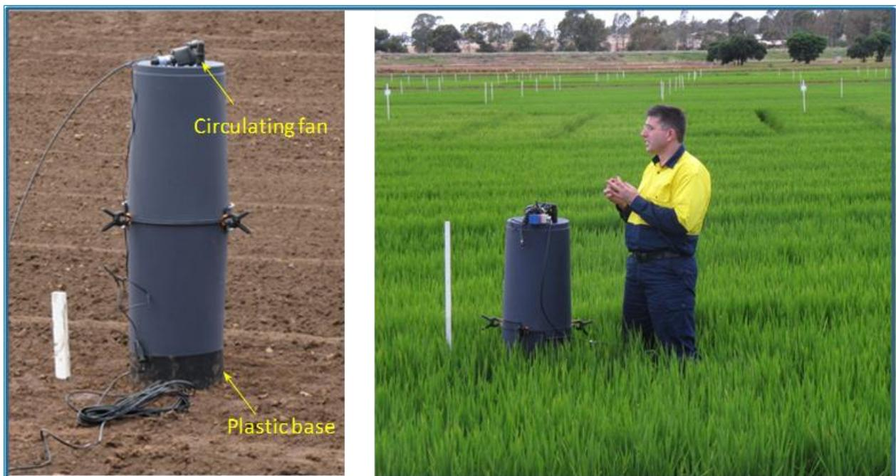
Figure 5.8. Purpose-built flux chamber used for measuring CH<sub>4</sub> emissions from rice
