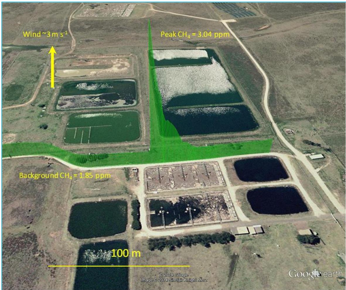
**Figure 6.39. Methane plume (shown as the green trace) detected during a downwind traverse of the effluent ponds at the Singleton wastewater treatment plant.**
