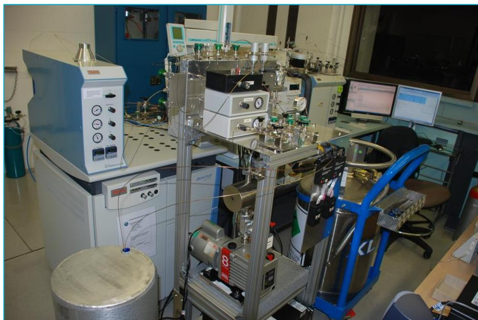
Figure 8.8. Photograph of the prototype cryogenic trap module
