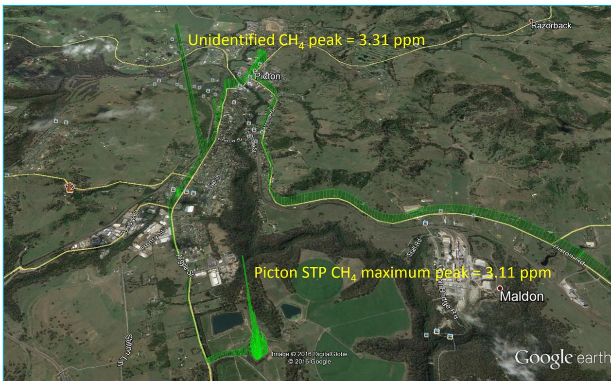
**Figure 6.46. Mobile survey of the Picton wastewater treatment plant and surrounding area made on 6<sup>th</sup> August 2014. Note the unidentified peak of CH<sub>4</sub> unrelated to the facility located near Picton.**
