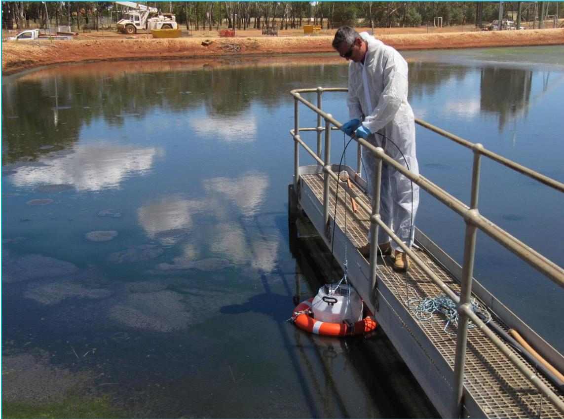
**Figure 6.44. Flux chamber measurements on one of the biosolids lagoons at Dubbo STP. Gas bubbles are visible on the surface of the lagoon.**
