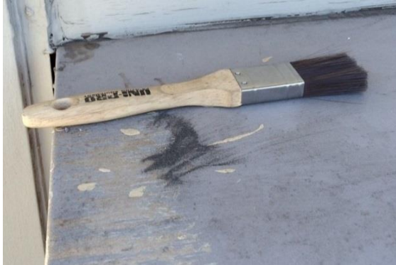
Figure 2 Typical Brush sample location and collection of dust sample which appears as black dust to the human eye.
