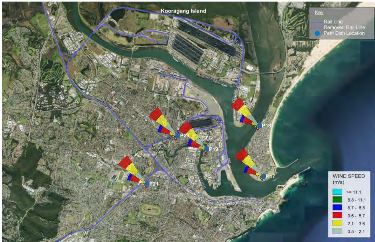
Figure 35: Wind Rose Overlay for Petri Dish Samples P17, P18, P19, P20 and P21
