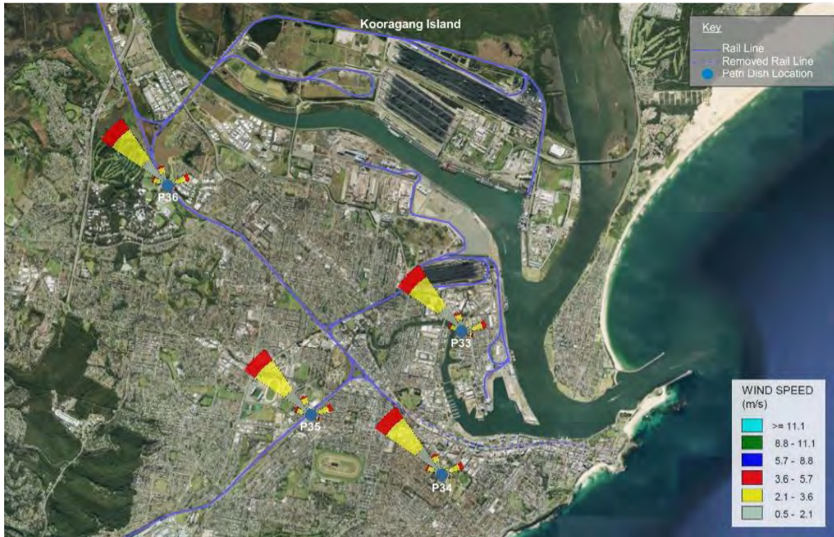
Figure 41: Wind Rose Overlay for Petri Dish Samples P33, P34, P35 and P36
