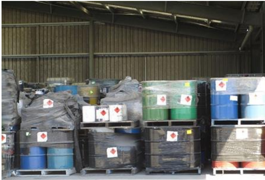
Good practice - all flammables stored together
