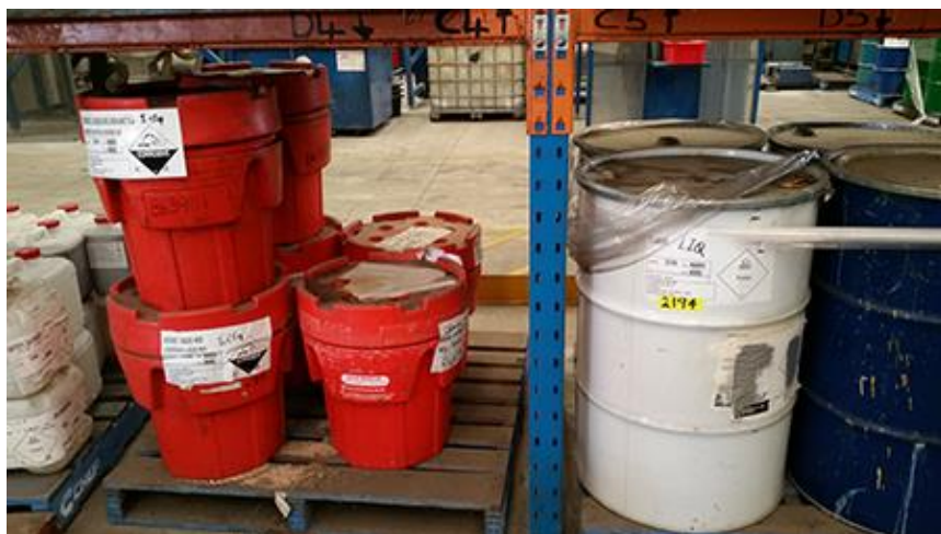
Bad practice - Class 8 Corrosive Acid stored next to Class 6 Toxic Cyanide
