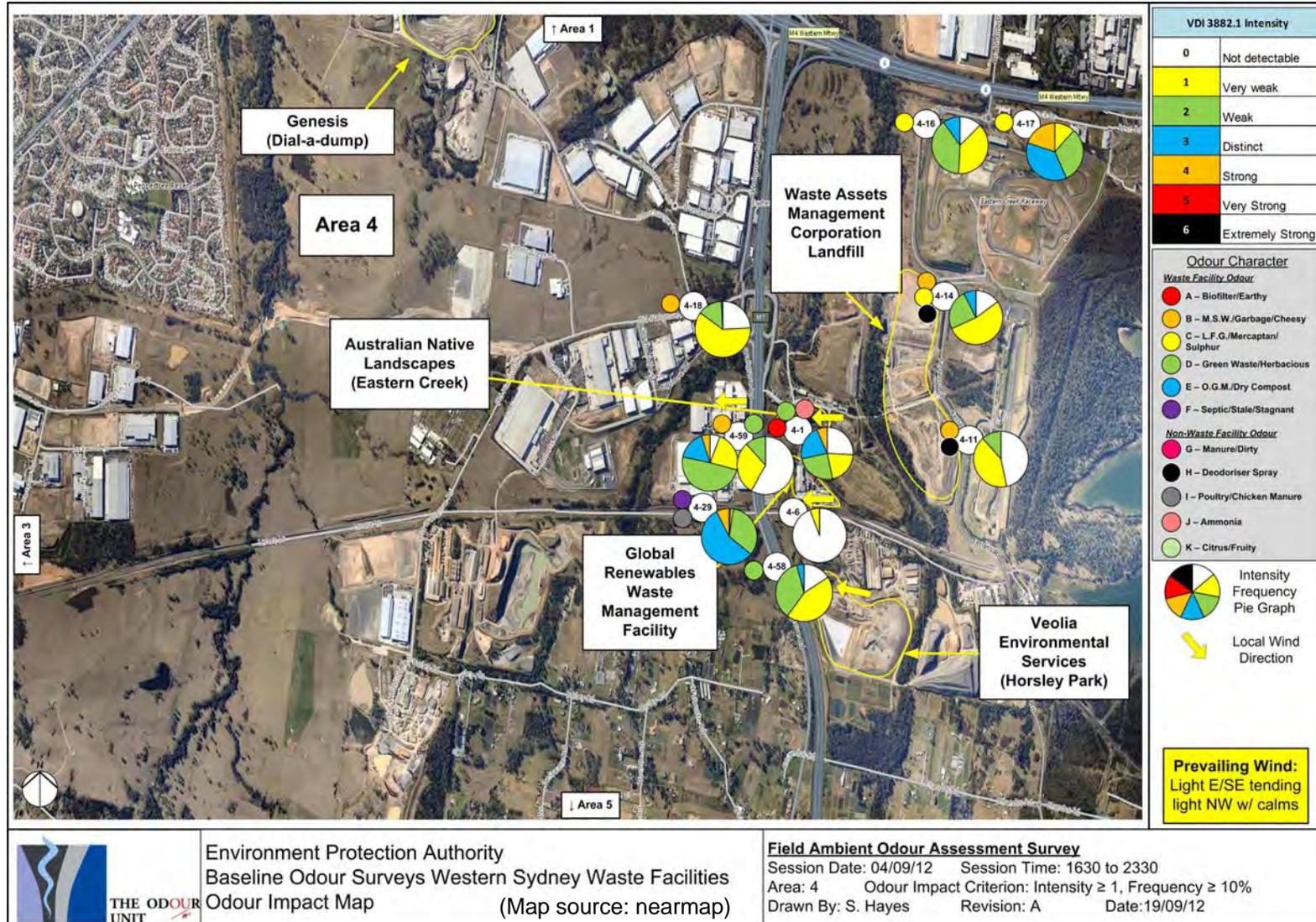
Figure 3.9 – An example of a survey map plot result showing 11 discrete measurements in Assessment Area 4
