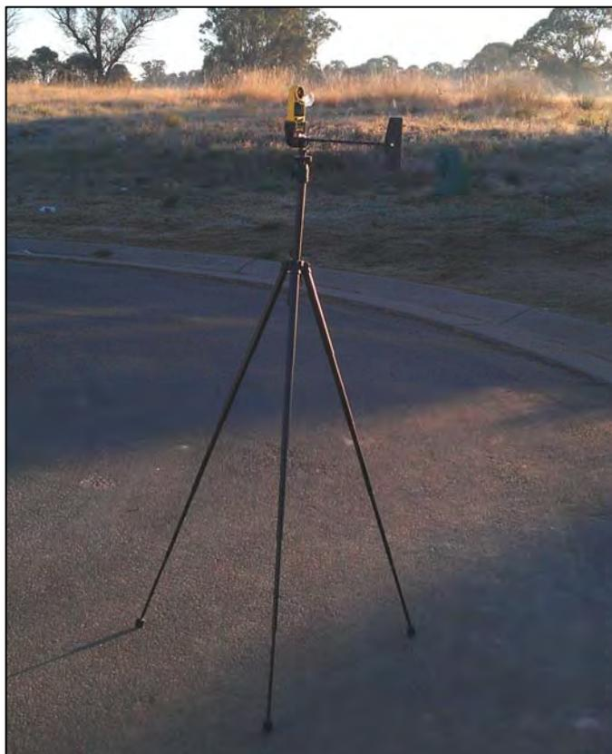
**Photo 3.1** – Kestrel Anemometer apparatus in operation (Source: The Odour Unit Pty Ltd)
