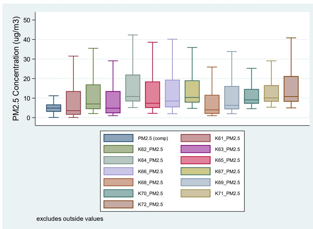
**Figure 5: Comparison of PM<sub>2.5</sub> readings for KOALA sensors Versus Compliance Station, 16-28<sup>th</sup> April 2019**
