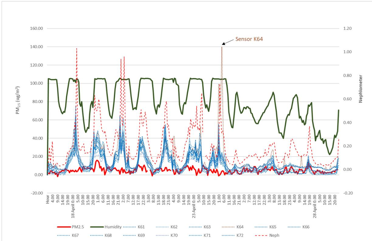
**Figure 6: Comparison of Real-Time PM<sub>2.5</sub> Measurement by KOALAs Versus Compliance Station, 16<sup>th</sup>-28<sup>th</sup> April 2019**
