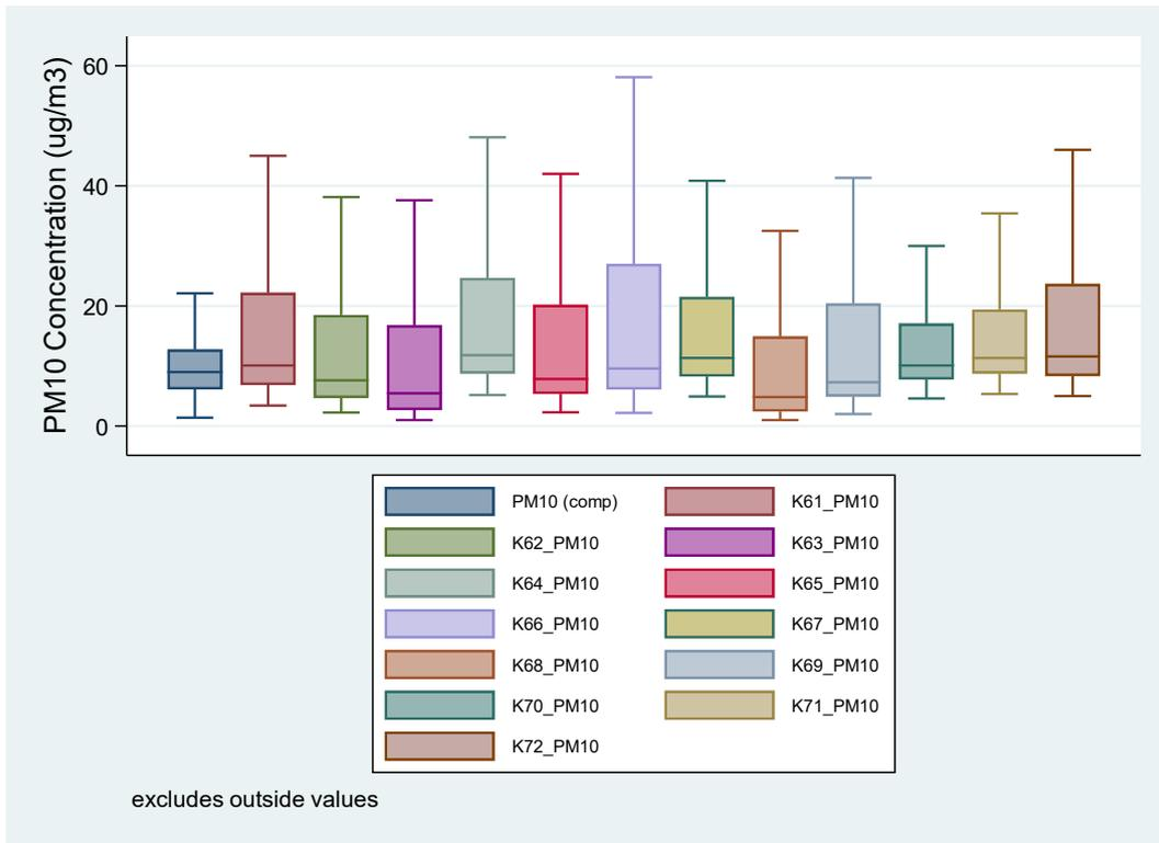
**Figure A1: Comparison of PM<sub>10</sub> readings for KOALA sensors Versus Compliance Station, 16-28th April 2019**
