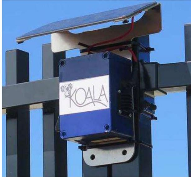
**Figure 1: KOALA low cost air monitoring sensor (QUT)**
