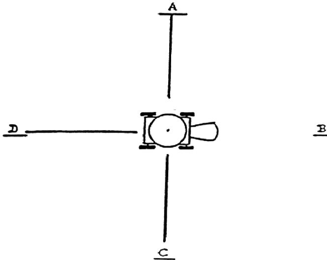
Figure 1: Typical test-site layout and microphone positions: grass-cutting machines (plan view)
