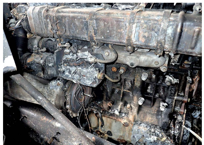
An engine bay after a fuel fire
