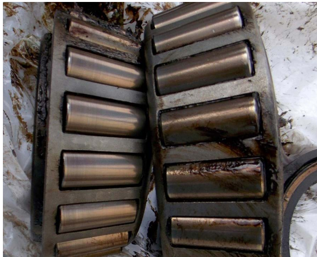
New bearings can be over-tightened. Blackened grease indicates hot bearing conditions. Photo: Peter Hart/Hartwood Consulting
