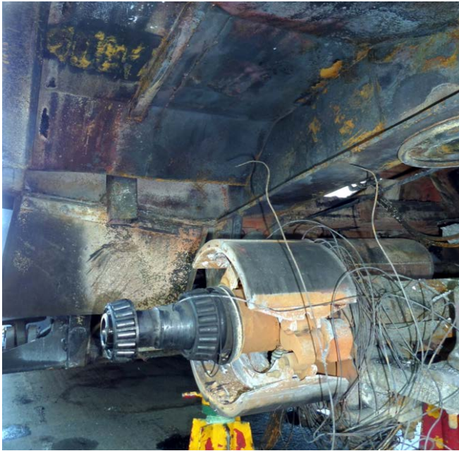
A tyre fire that resulted from a deflated air suspension. The tyre rubbed on the metal guard, causing the tyre tread to overheat. Photo: Peter Hart/Hartwood Consulting
