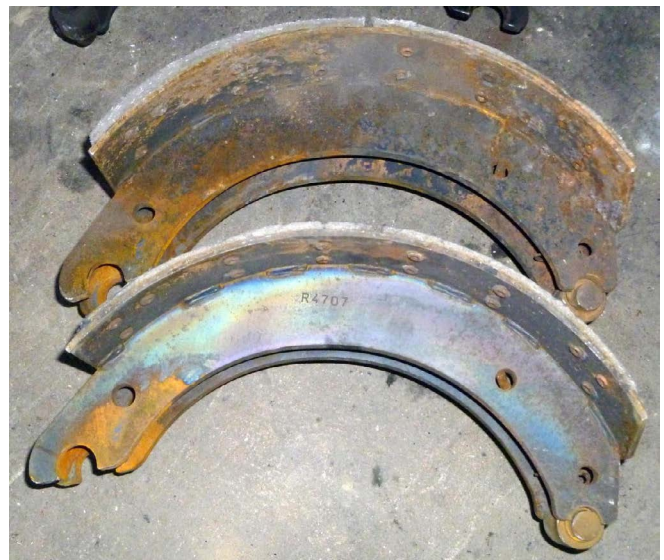
Rubbing brakes cause extreme brake temperature. Photo: Peter Hart/Hartwood Consulting
