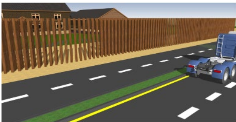
Figure 73 Example of a sonic crystal-type barrier (Amado-Mendes et al., 2016).
