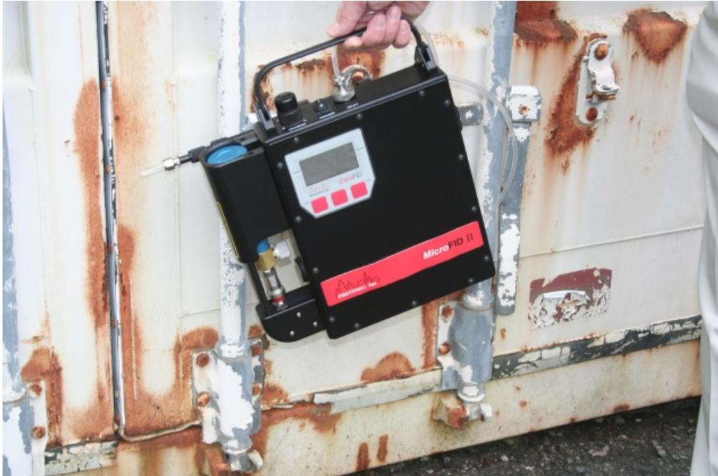
Figure 19 Infinicon/Photovac’s MicroFID II
