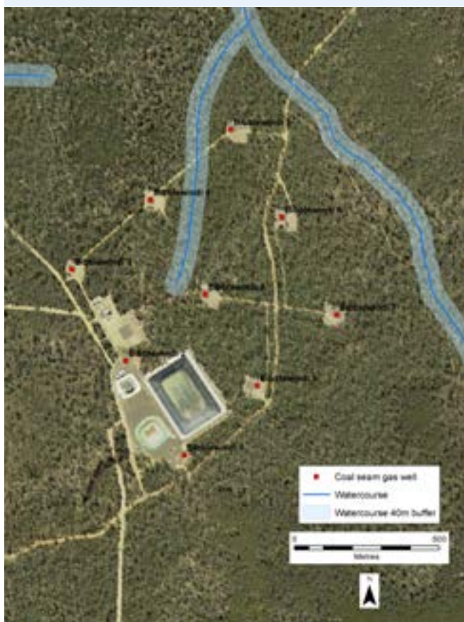
Remote sensing image of Bibblewindi gas wells. Red dots indicate the wells, blue shaded areas show the 40 metre buffer zones. Image courtesy of Department of Finance, Services & Innovation
