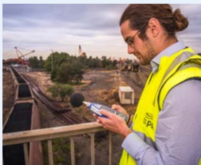
Hunter EPA CareerTracker Marshall Sing assessing coal train pass-by noise levels. Photo: John Spencer/EPA
