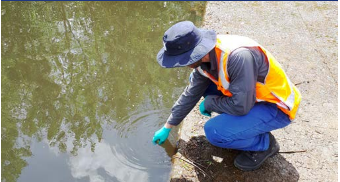
EPA officer collecting water sample to assess impact of a sewage overflow on the waterway.
