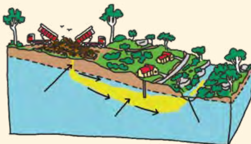
Contamination of groundwater from dumped rubbish
