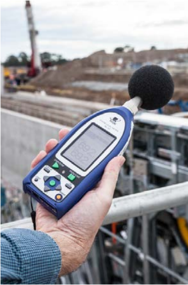
Noise monitoring at a construction site. Photo: Sarah Ryan/EPA
