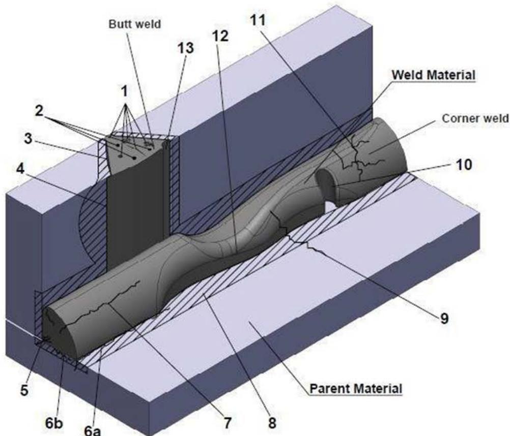
**1. Fine/Coarse Cluster Porosity/blow holes & hollow root beads:**
