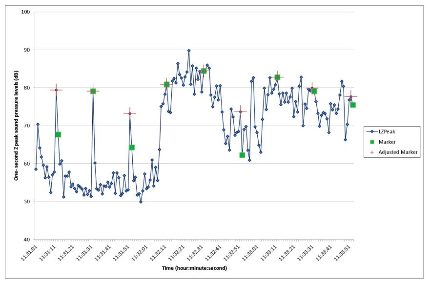
Figure 1: Sequence of one-second Z peak levels (decibels (dB)), markers, and markers adjusted for likely delay between the measurement attendant hearing the shot and placing the marker.
