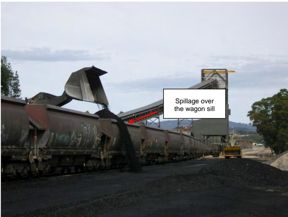
**Stationary loading: Front-end loader for loading of stationary train (top) and spillage of coal over the wagon sill during loading (bottom) (photo: E Howard (top)/ T Greyling (bottom))**
