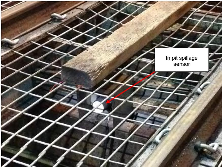
**Controls to prevent spillage from the bottom of coal wagons: White markings on door closing mechanism to identify open doors (top) and in-pit spillage sensor at a coal load-out facility (bottom) (photo: L Silk (top)/ T Greyling (bottom))**
