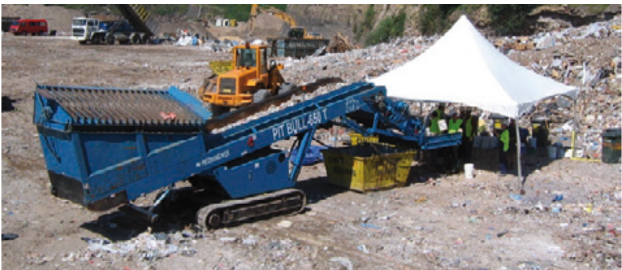
Photograph 3 – Pitbull screening plant with picking belt, for manual sorting
