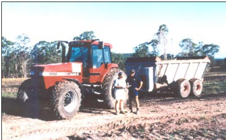
Plate 6.2 Tractor drawn manure spreader used for the application of compost.
