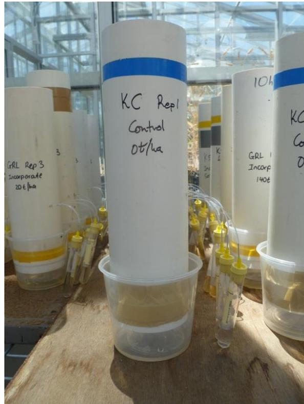
**Figure 7.8. Set up of one soil column with the plastic container at the bottom to collect leachate and pore water samplers at 15 cm.**
