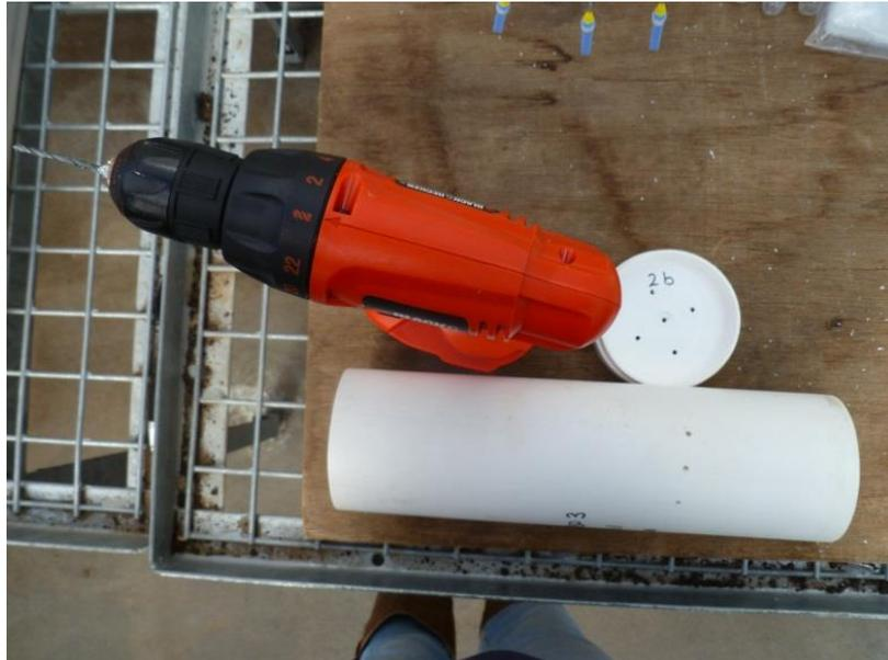
**Figure 7.5. Drill holes in the caps for the bottom of the soil columns and the side of the columns for the pore water samplers.**
