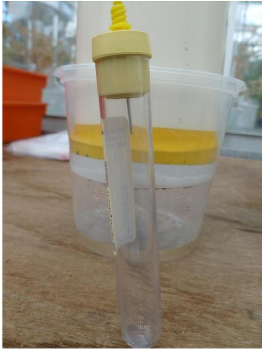
**Figure 7.7. The BD Vacutainer Urinalysis Plus Urine Tubes used to collect leachate at 15 cm from the pore water samplers.**
