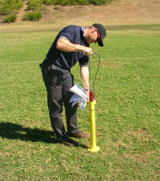
Figure 5. Clegg hammer impact testing of surface hardness on Ched Towns Oval.
