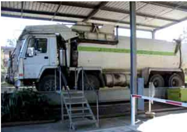
Photo 24.2 Commercial vehicle being weighed on entry
