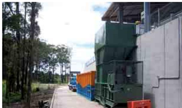
Photo 14.5 Stationary compactor and transfer container
