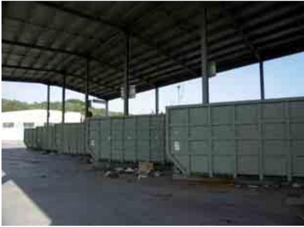
Photo 19.4 Skip bins located at the transfer station
