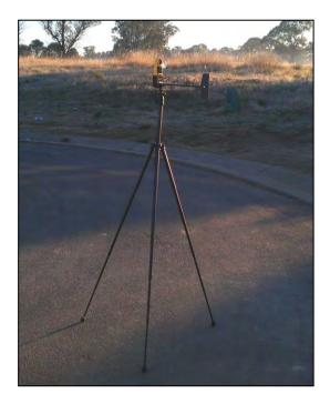
**Photo 4.1** – Kestrel Anemometer apparatus in operation
