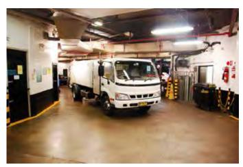
Figure 21 Small vehicle for access to areas with low clearance
