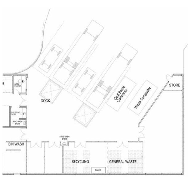
Figure 54 Example loading dock design
