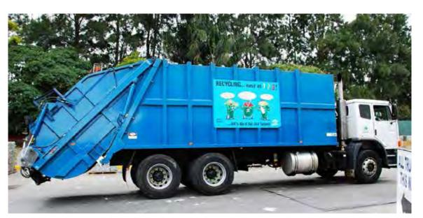
Figure 57 A rear-lift collection vehicle
