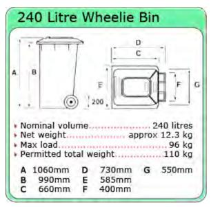
Figure 35 Typical 240 litre capacity bin specifications
