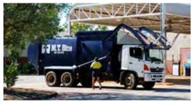
Figure 29 Front-lift truck
