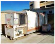
Figure 28 Transportable compactor
