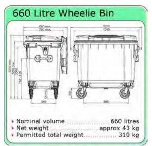
Figure 37 Typical 660 litre bin specifications
