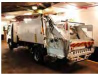
Figure 31 Rear-lift collection vehicle
