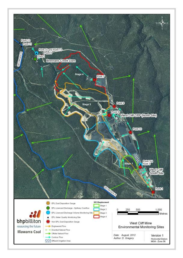
Figure 1-1: West Cliff Colliery Site Plan showing Brennans Creek dam and EPL 2504 water discharge and quality monitoring points
