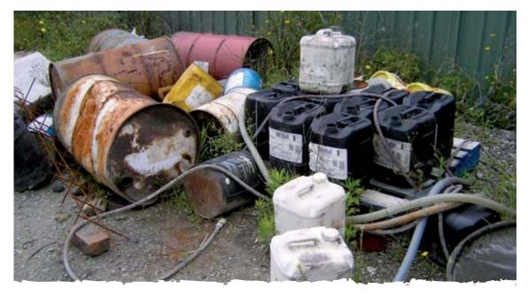
Batteries and chemicals should not be stored without containment (DECC)
