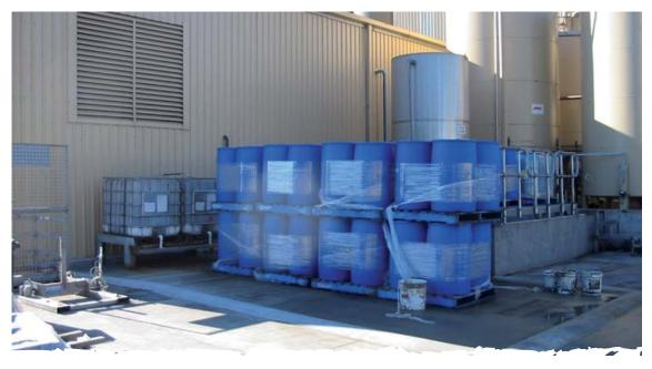
Storing chemicals properly, with appropriate containment, prevents spills and leaks from escaping (DECC)
