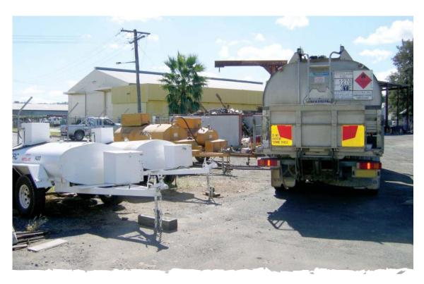
Filling mobile tankers without containment is dangerous (DECC)
