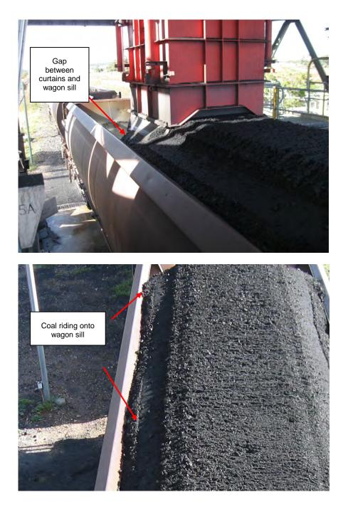
Worn out or poorly calibrated profiling curtains (top) resulting in coal 'riding up' onto wagon sills (bottom) (photo: L Silk (top/bottom))
