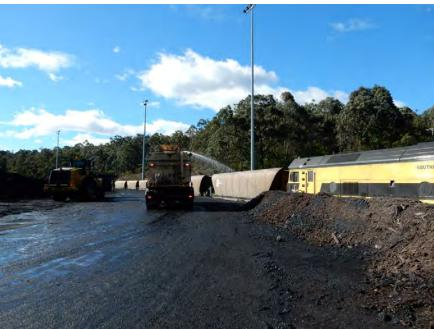
Good practices: removal of coal from wagon gunnels by means of the gunnel brush (top) and use of a water jet to remove coal from wagon exteriors (bottom) (photo: W Wickremeratne (top)/ M Karam (bottom))
