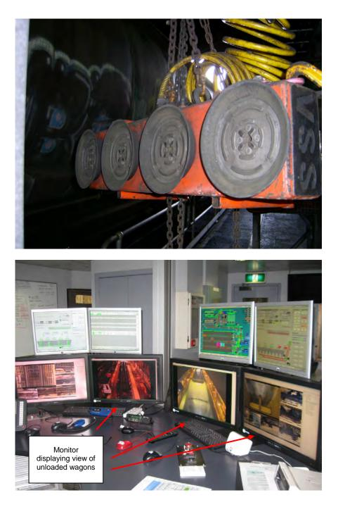
Magnetic vibration device to dislodge hung up coal (top) and control room displays showing the interior of unloaded wagons to monitor for potential carry back coal (bottom) (photo: L Silk (top)/ R Deves (bottom))
