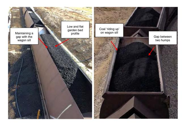
Loading coal with a low, flat garden bed profile (left) as opposed to an uneven, undulating profile minimises coal losses from the tops of wagons (photo: E Howard (left)/ W Wickremeratne (right))
