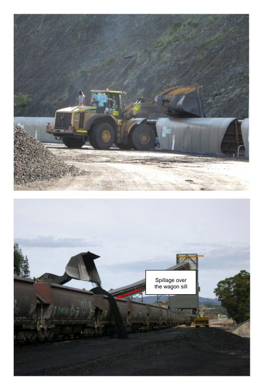
Stationary loading: Front-end loader for loading of stationary train (top) and spillage of coal over the wagon sill during loading (bottom) (photo: E Howard (top)/ T Greyling (bottom))
