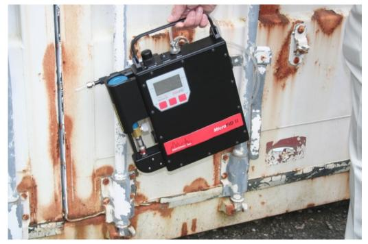
Figure 19 Infinicon/Photovac's MicroFID II
