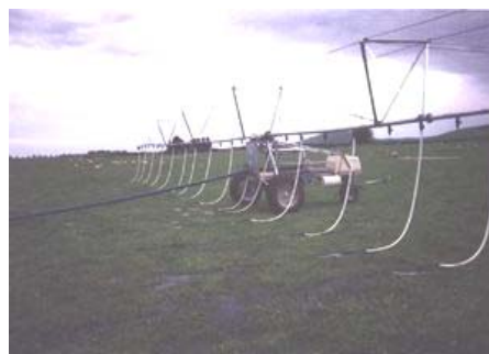
Traveling effluent irrigator with droppers
