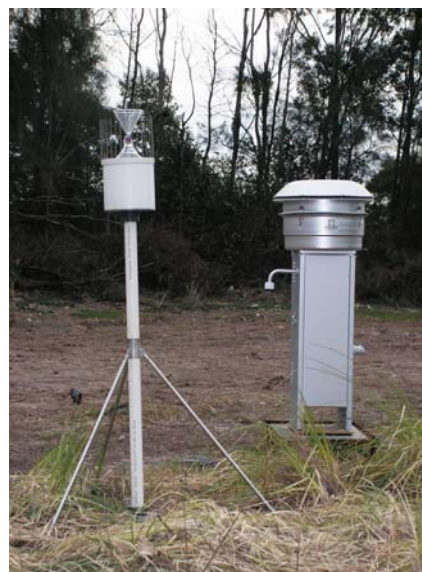
Air pollution monitors on a construction site
