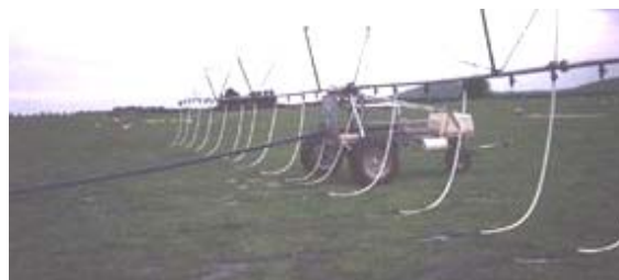
Travelling effluent irrigator with droppers
