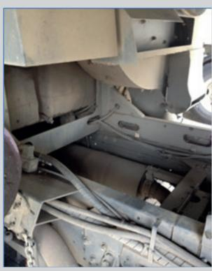
Figure 4: Partial Diesel Particulate Filters fitted to a Blacktown City Council street sweeper; main and stationary engine. Photo: John Bannister, Blacktown City Council
