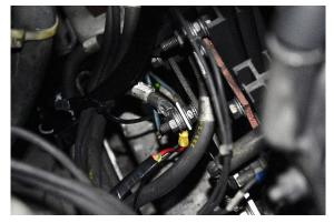
Voltage connections for auxiliary DC generator
