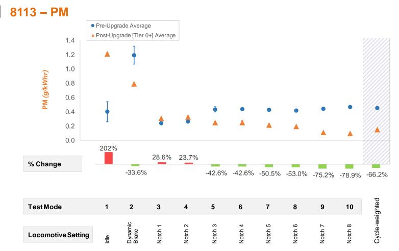
PM emissions increased after installation of the emissions upgrade kit in modes 1, 3 and 4, by 23.7% to 202%. In all other modes, PM was significantly reduced by between 33.6%, in dynamic brake and 78.9%, in notch 8 when compared to the standard engine rebuild results.
