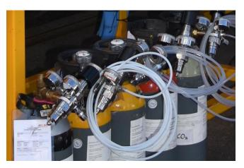
PEMS calibration includes a leak check, gaseous calibration with certified gas and data check.
