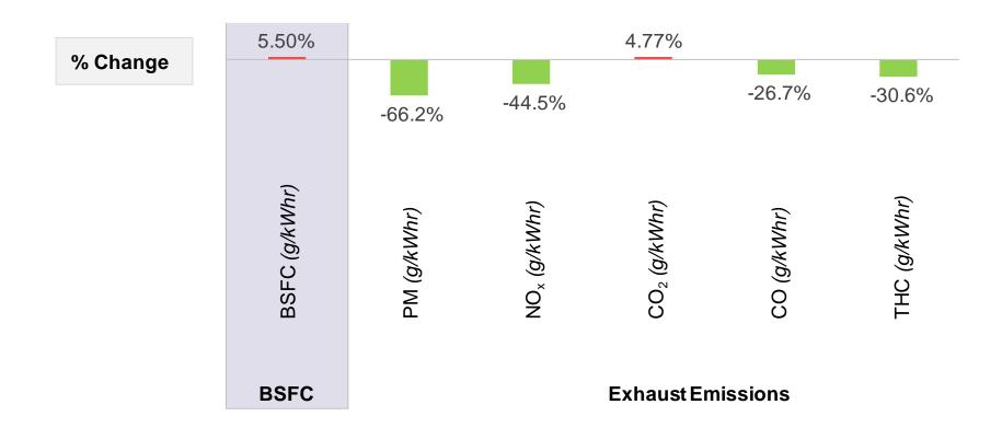
Significant reductions in particulate and regulated gaseous emissions were achieved in the cycle weighted emissions results after the installation of the Tier 0+ engine emissions kit. BSFC results have been corrected for temperature and humidity as per the Association of American Railroads (AAR) practice, whereas emissions results are uncorrected. For this reason, there is a difference between the percentage change in BSFC and CO2 presented within the report.
