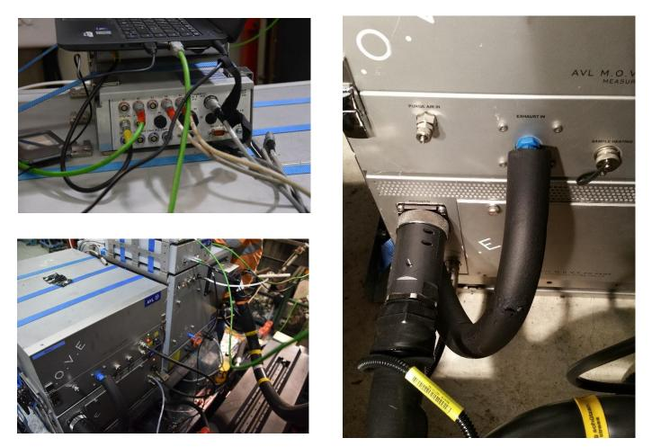
Warm up PEMS before calibration and test. Approx 60 minutes. Gaseous sample line to 191°C and PM sample line to 52°C.
