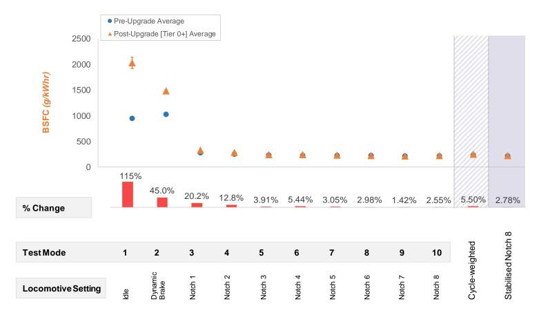
The change in BSFC between test configurations was lowest in the higher notches. Percentage change in BSFC ranged between 1.42% in notch 7 to 115% in idle. The test to test repeatability in both pre and post emissions upgrade configurations was excellent, and within 1%, with the exception of modes 1 and 2 which varied between 1.78% and 10.4%.
