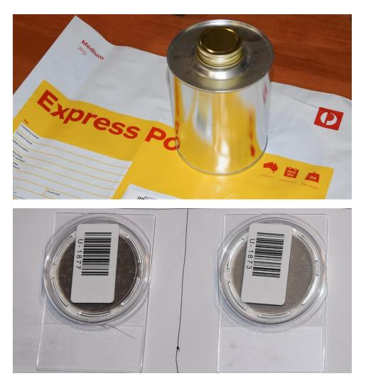
Send diesel fuel sample and gravimetric filters for analysis.
