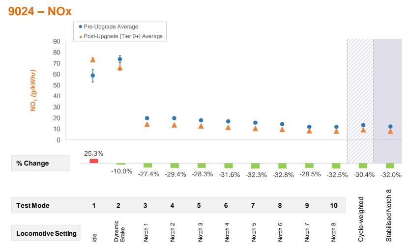
NOx emissions improved significantly after the installation of the upgrade kit with cycle weighted NOx emissions reducing by 30.4%. NOx was significantly reduced by between 10.0% in dynamic brake and 32.8% in notch 6 when compared to the standard engine rebuild results.
