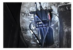
Voltage transducer on main DC generator
