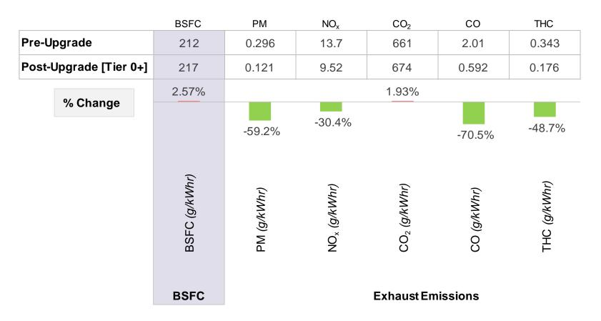
Significant reductions in particulate and regulated gaseous emissions were achieved in the cycle weighted emissions results after the installation of the Tier 0+ engine emissions kit. An increase in the BSFC with the upgrade kit installed, indicates lower engine efficiency.
