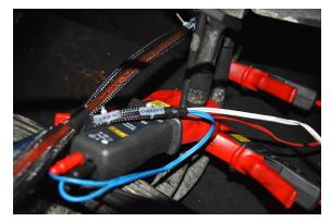
Current clamps on companion AC alternator cables
