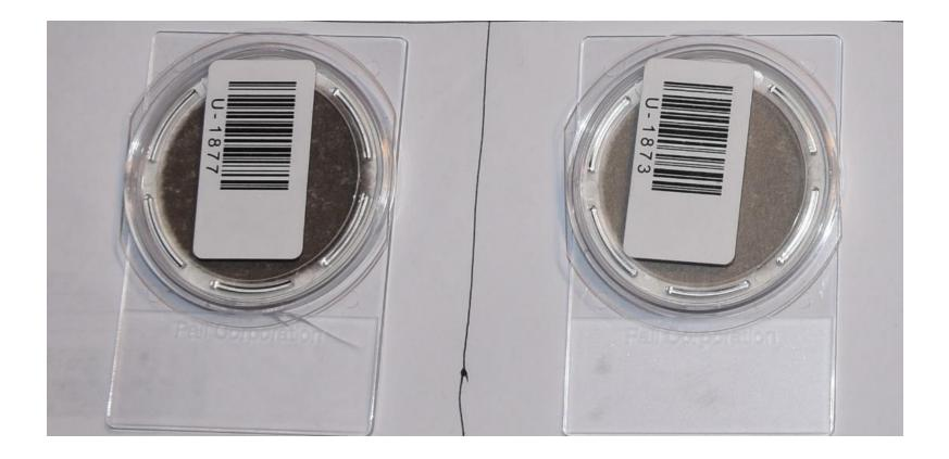
New filter for each test mode [10 per test]
