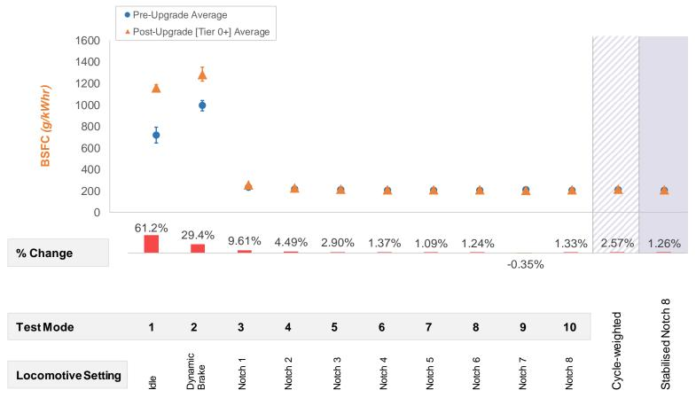
The change in BSFC was lowest in the higher notches. Percentage change in BSFC ranged between 1.09% in notch 5 to 61.2% in idle. Overall, the test to test repeatability in both pre and post emissions upgrade configurations was very good.
