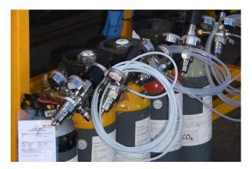
PEMS analyser drift check, leak check and data check.
