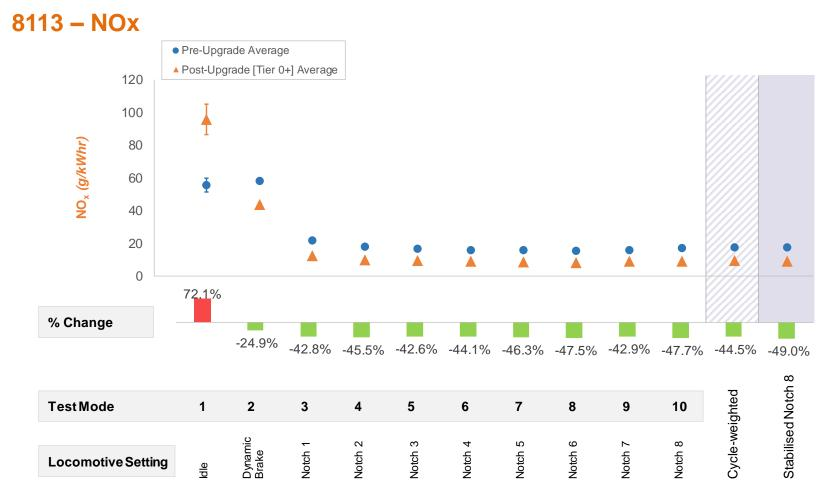
NOx emissions increased after installation of the emissions upgrade kit only in mode 1 (idle), by 72.1%. In all other modes, NOx was significantly reduced by between 24.9%, in dynamic brake and 47.7%, in notch 8 when compared to the standard engine rebuild results. Test to test repeatability was excellent, typically within 1%, with the exception of testing in mode 1.
