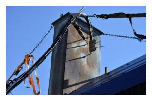
Exhaust stack and emissions sample probes on 8113
