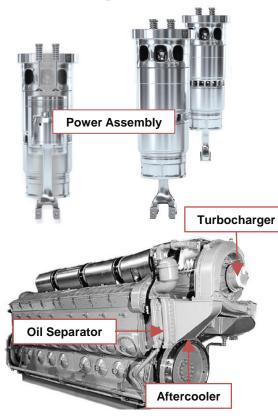
**Ultra Low Lube Oil Power Assembly** - The introduction of a hardened upper bore liner with specially designed bore profile and piston crown with improved piston ring design results in a claimed reduction in oil consumption by 50%.
