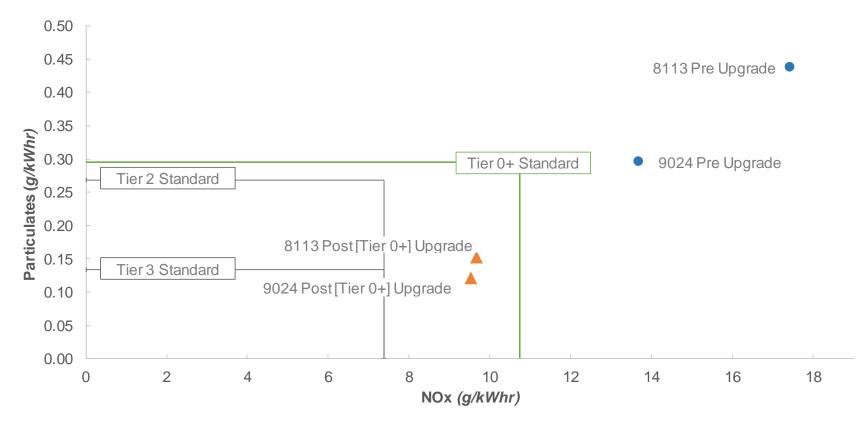
When compared to the Tier 0+ emissions limits, 8113 achieved reductions of 48.3% and 9.95% for PM and NOx respectively, whilst 9024 achieved reductions of 59.1% for PM and 11.2% for NOx.
