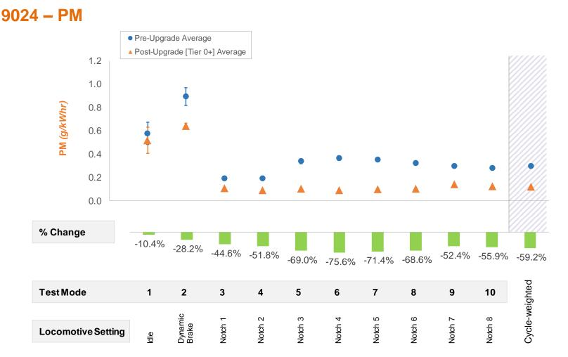
In all modes, PM was significantly reduced by between 10.4%, in idle and 75.6%, in notch 4 when compared to the standard engine rebuild results. The greatest improvements in PM emissions were measured in notch 3 to 5.
