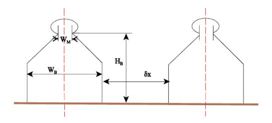
Figure 3-3. Shows a cross-section of two adjacent buildings with dimensions defined (Schulman and Scire, 1980). The GUI screen shot below from CALPRO shows the Line Source Input section.
