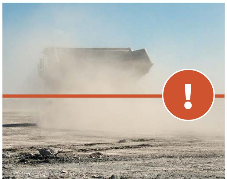
This series of photos shows dust levels with and without the application of water to the haul road.
