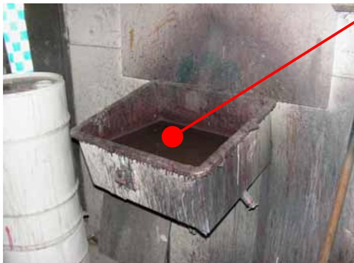
Here all used solvents and the washings from painting equipment have simply been put into an open container in the workshop with no method of containing the vapours.
