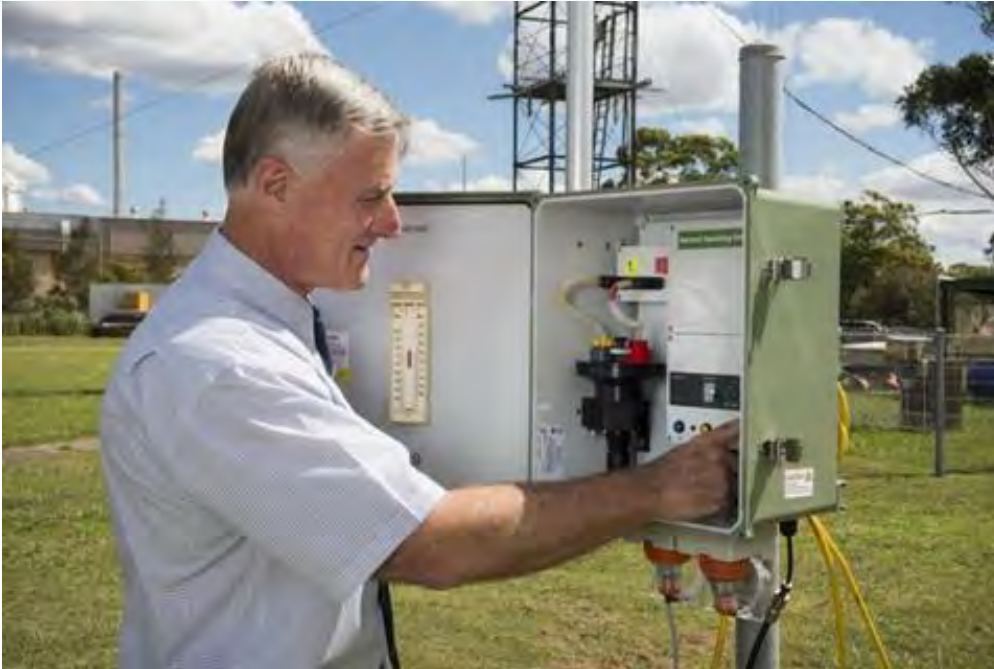
PM2.5 Cyclone unit with its microprocessor at Lucas Heights
