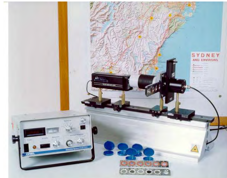
Black carbon laser instrument
