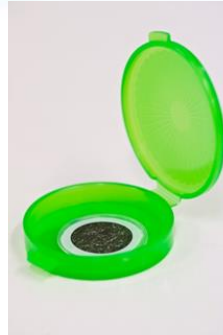
Exposed stretched Teflon filter, specifically design for IBA analysis
