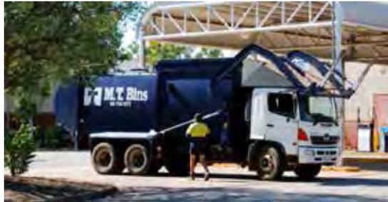
Figure 29 Front-lift truck
