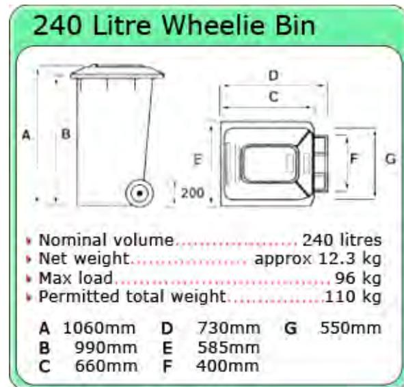
Figure 35 Typical 240 litre capacity bin specifications
