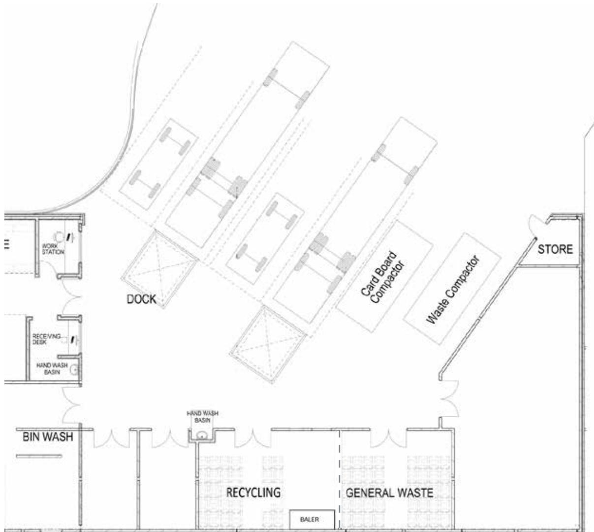
Figure 54 Example loading dock design
