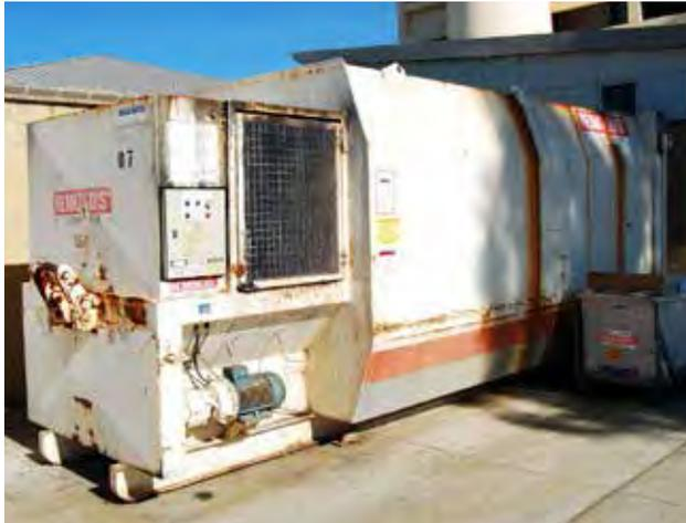
Figure 45 Integrated waste compactor
