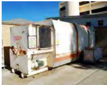
Figure 28 Transportable compactor
