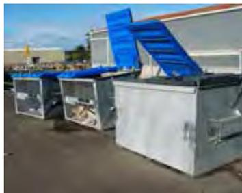
Figure 25 Front-lift bulk bins for cardboard (left) and garbage (right)
