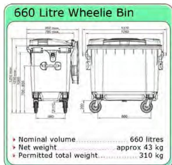
Figure 37 Typical 660 litre bin specifications
