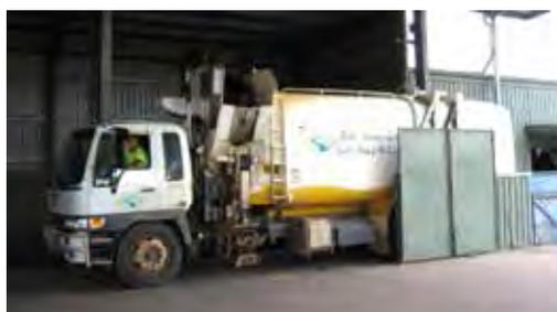
Figure 32 Side-lift collection vehicle
