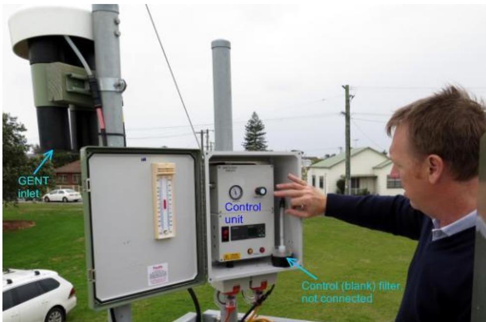
**Figure 19: Details of the GENT sampler at the Stockton site being inspected by Peter Crabbe**
