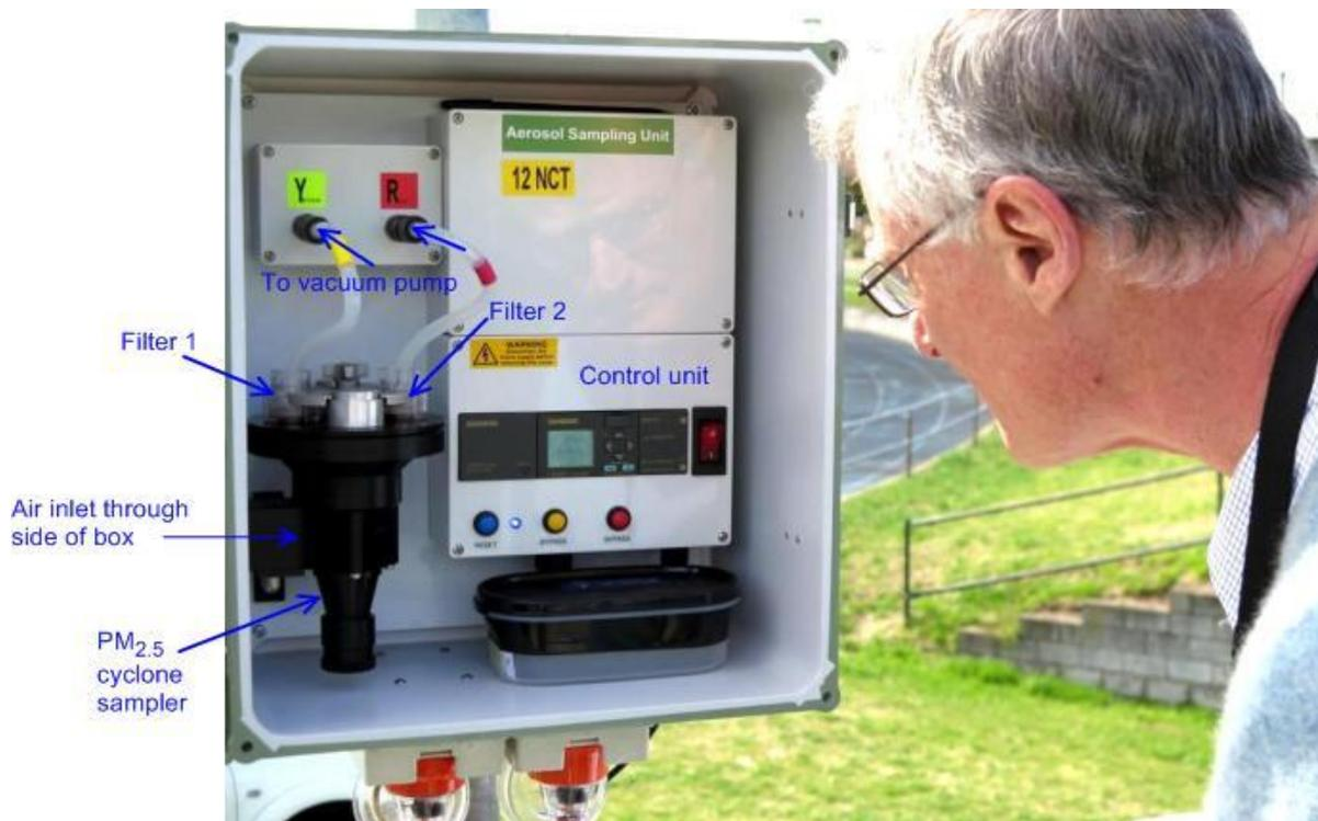
Figure 17: Details of the ASP Sampler at the Newcastle site being inspected by David Cohen
