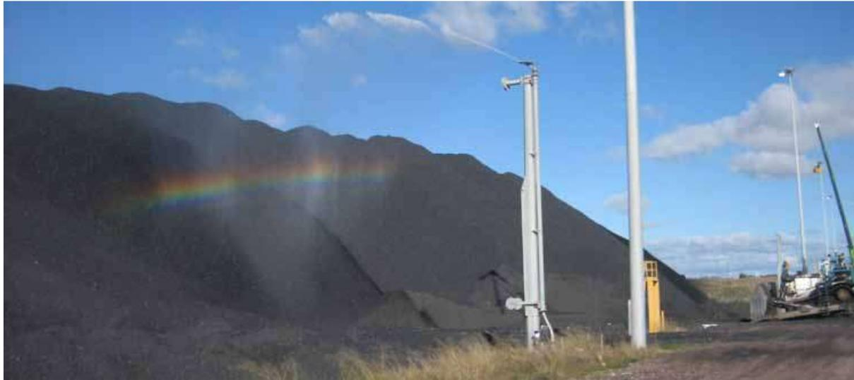
**Figure 57 Stockpile sprays**
