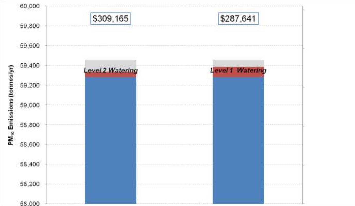
**Figure 66 Reduction in emissions and associated costs (per tonne) to implement control options on grading**
