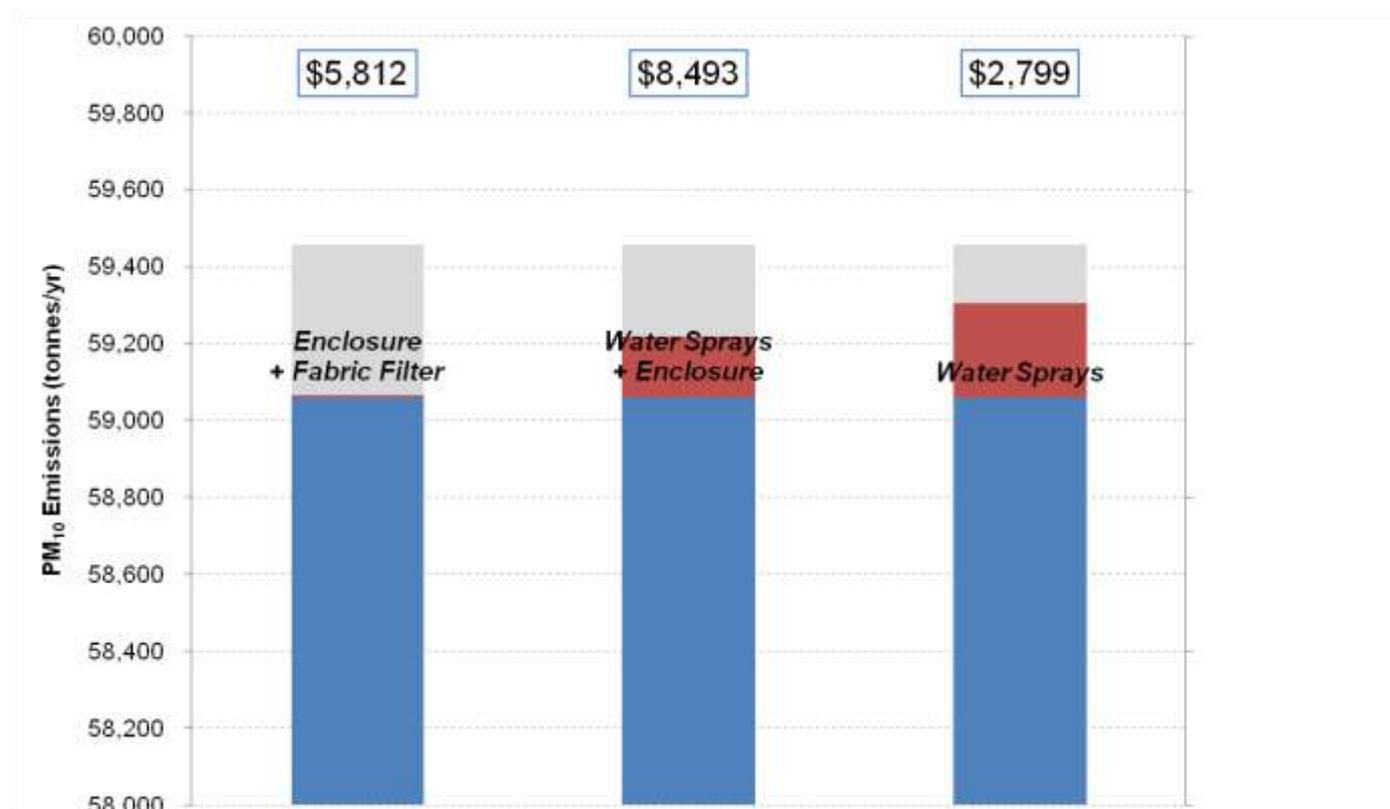
**Figure 65 Reduction in emissions and associated costs (per tonne) to implement control options on trucks dumping coal at the ROM hopper**
