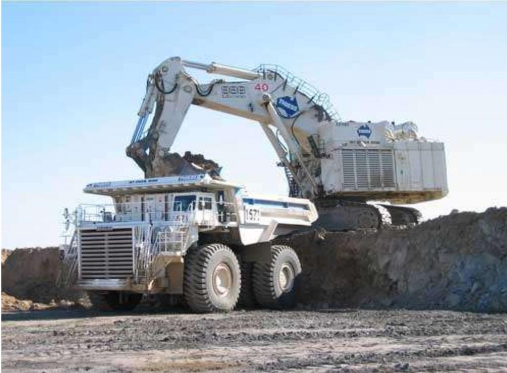
**Figure 6** Large excavator loading haul truck
