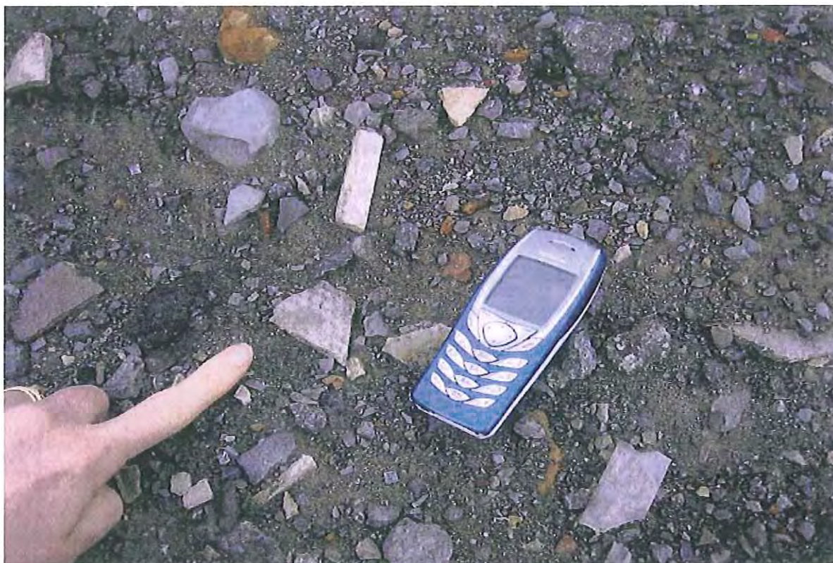
Figure 11 - Exposed pieces of broken asbestos bonded sheet at 79 Betts Road Smithfield
