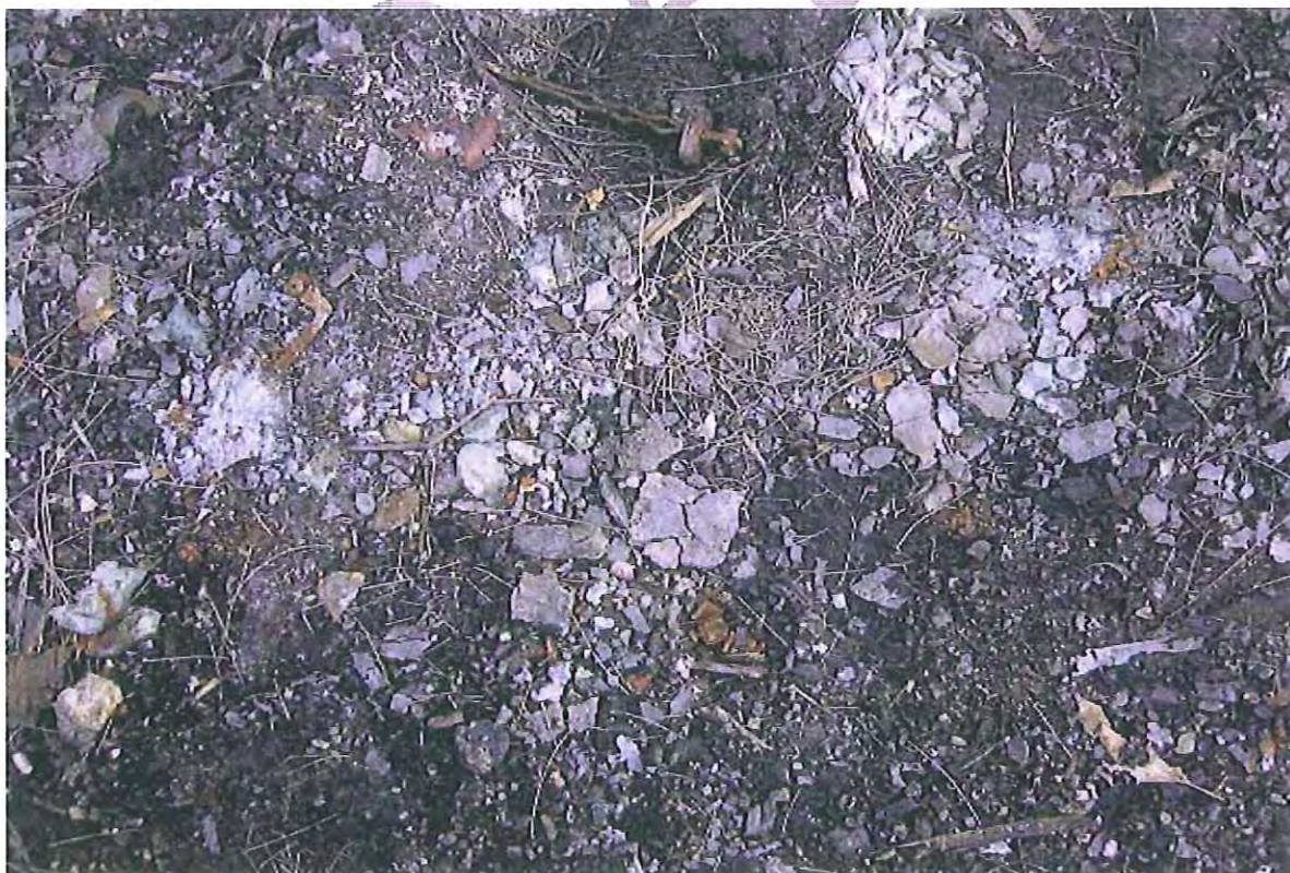
Figure 12 - Exposed pieces of broken asbestos bonded sheet at 79 Betts Road Smithfield
