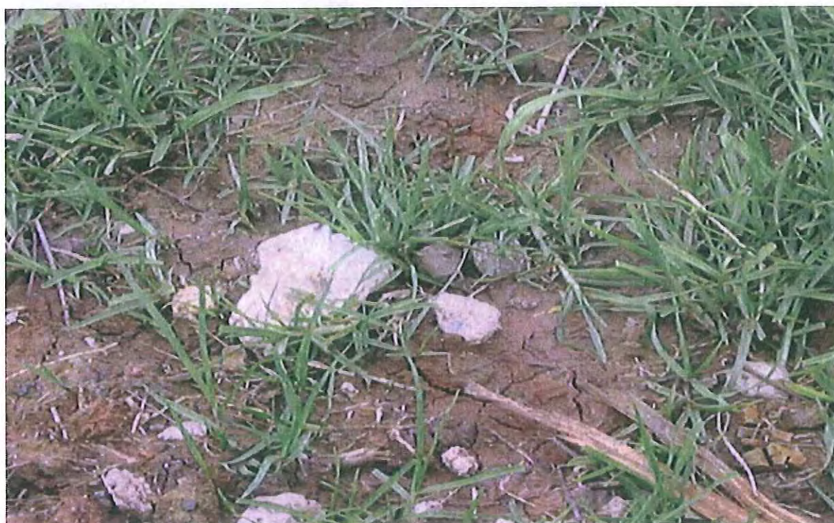
Figure 8 – Exposed pieces of broken asbestos bonded sheet at Old Clay Pit, Edensor Park
