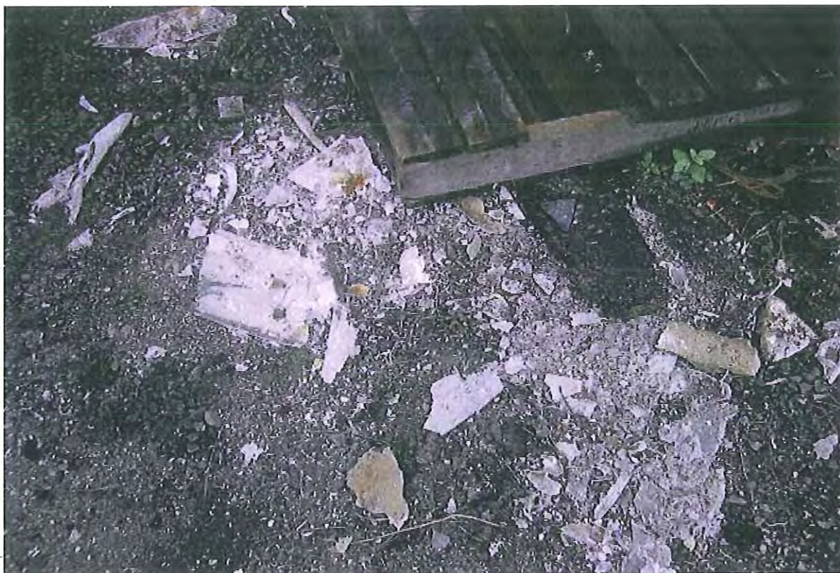
Figure 9 - Exposed pieces of broken asbestos bonded sheet at 79 Betts Road Smithfield
