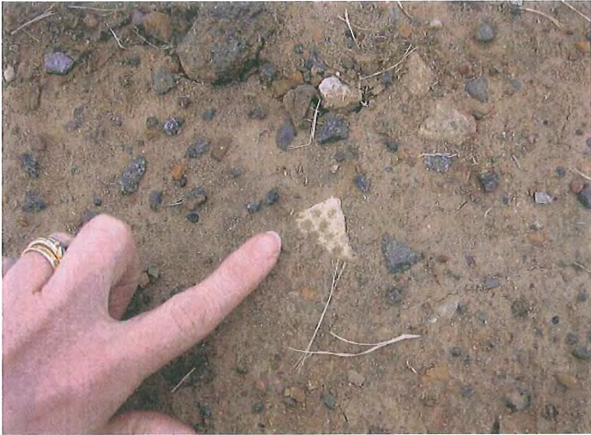
Figure 6 - Exposed pieces of broken asbestos bonded sheet at Hyland Road Park
