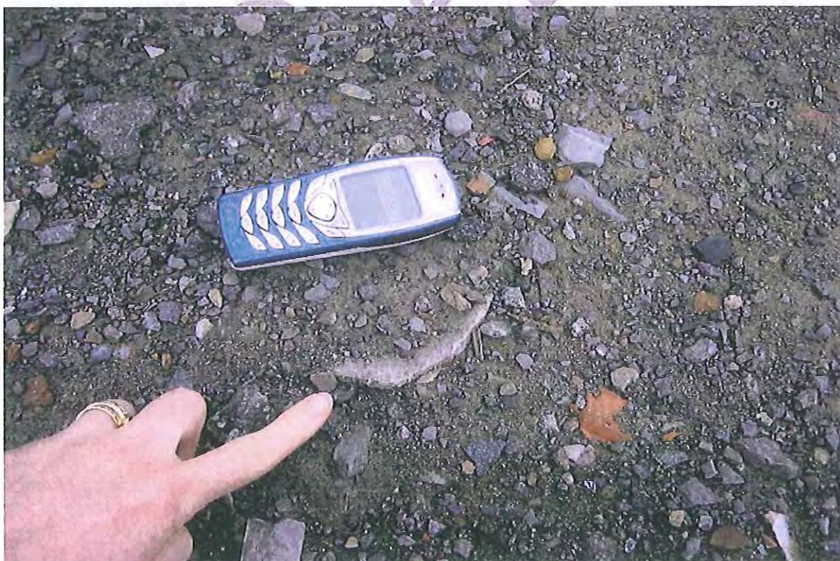
Figure 10 - Exposed pieces of broken asbestos bonded sheet at 79 Betts Road Smithfield
