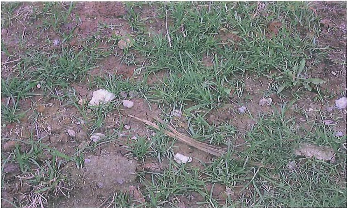
Figure 9 - Exposed pieces of broken asbestos bonded sheet at Old Clay Pit, Edensor Park
